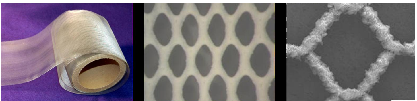
Figure 1: Microlith® mesh coated with sorbent.
