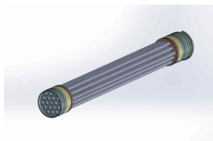
Figure 4: Potted module cross-section (left-most); new tube sheet module design (right).
