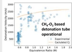
Detonations achieved with coal injection with  $CH_4$  and  $O_2$ . Visible images of tube exhaust provide evidence that coal is not completely combusted in the tube. The arrangement is in place to measure electrical conductivity in addition to detonation velocities.
