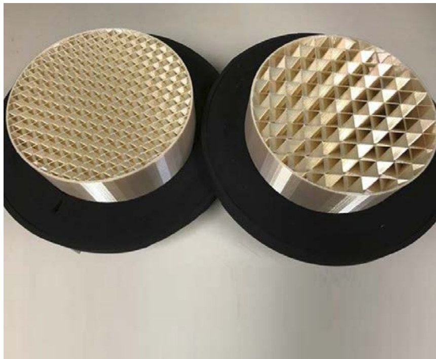
Figure 2: Packing with different cell densities, 3D-printed at ORNL.
