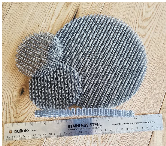
Figure 2: Froth-generating and -propagating screens.
