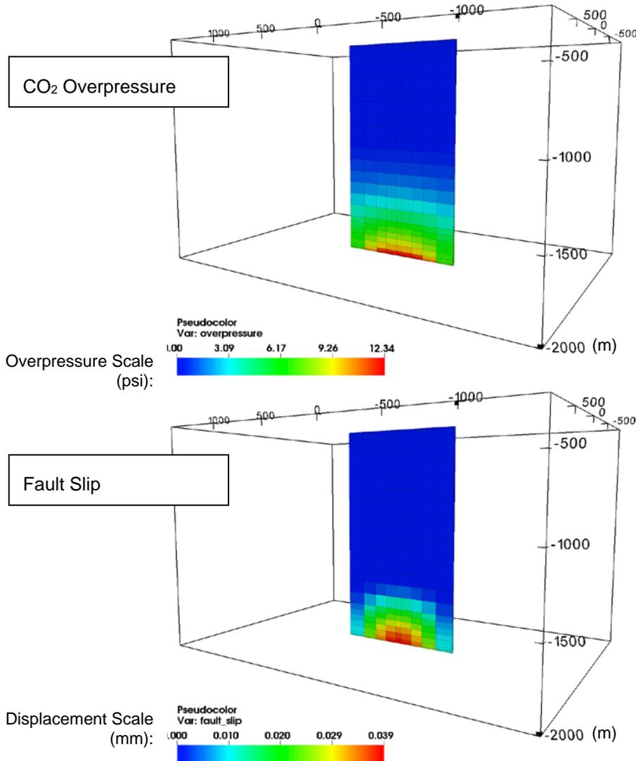
**Figure 1: Analysis results: A typical realization of the fault plane of leakage model. (Surrounding caprock is hidden, so that only the fault plane is visible.)**
