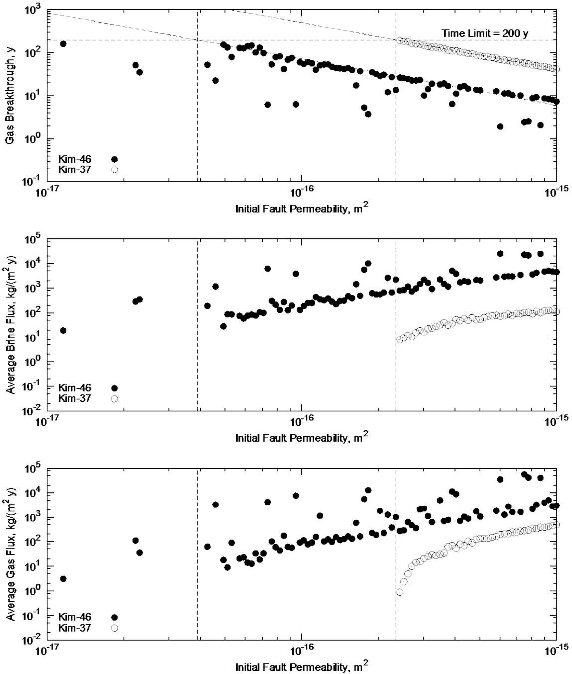
Figure 3: Fault leakage model results for two Kimberlina boundary models. Kimberlina 46 has the highest pressure distribution, while Kimberlina 37 has the lowest pressure distribution.
