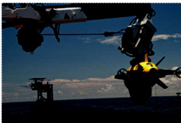
Marlin™ Launch prior to Platform Inspection
