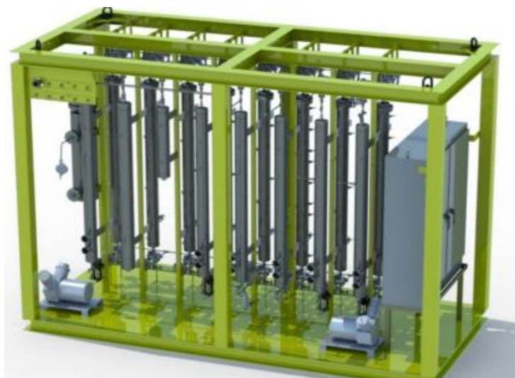
Figure 7: Eight-column integrated WGS and CO 2 capture unit.
