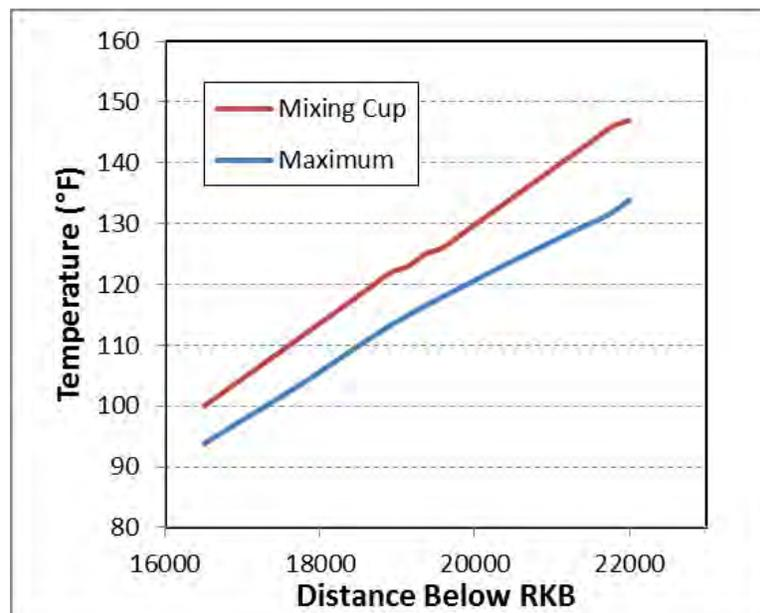
Figure 8. Temperature in the cement at the end of reverse placement.
