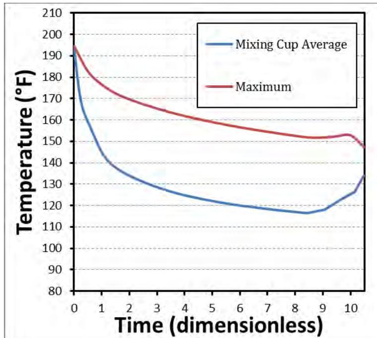
Figure 7. Bottom Hole Circulating Temperature during reverse placement
