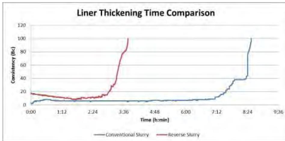
Figure 10: Thickening time of a 16'' liner slurry, 14,000' MD
