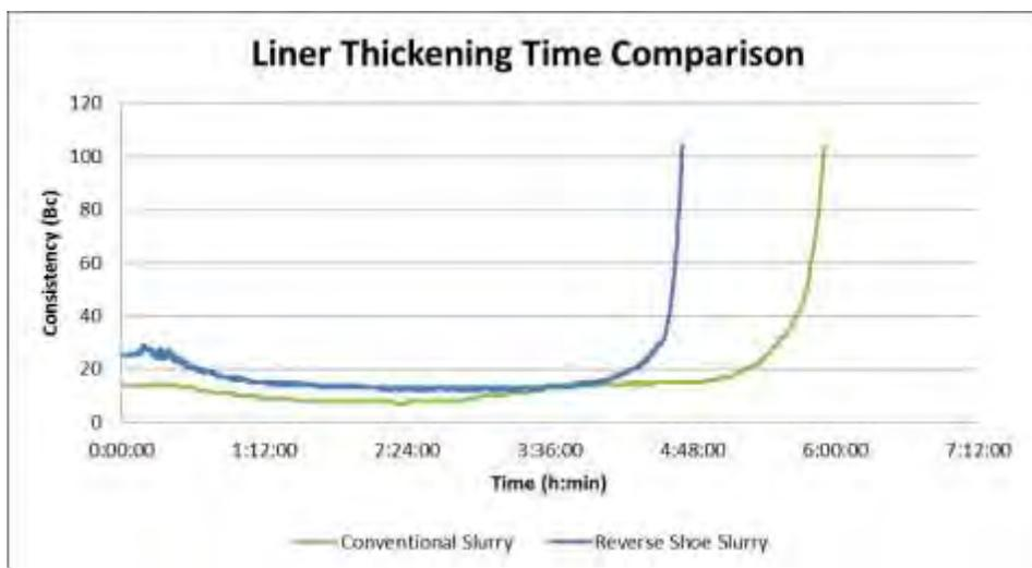
Figure 11: Thickening Time of an 11 7/8" Liner slurry, 24,000' MD
