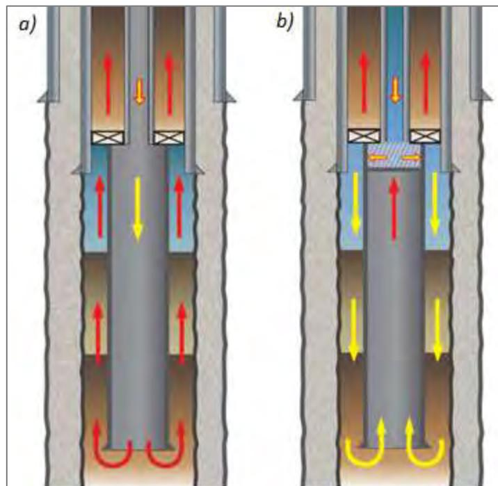
Figure 1: Flow path of fluids during conventional placement (a) and reverse placement (b) in a deepwater liner
