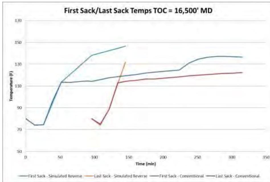
Figure 9: Comparison of simulated reverse and conventional 16'' liner temperatures during placement
