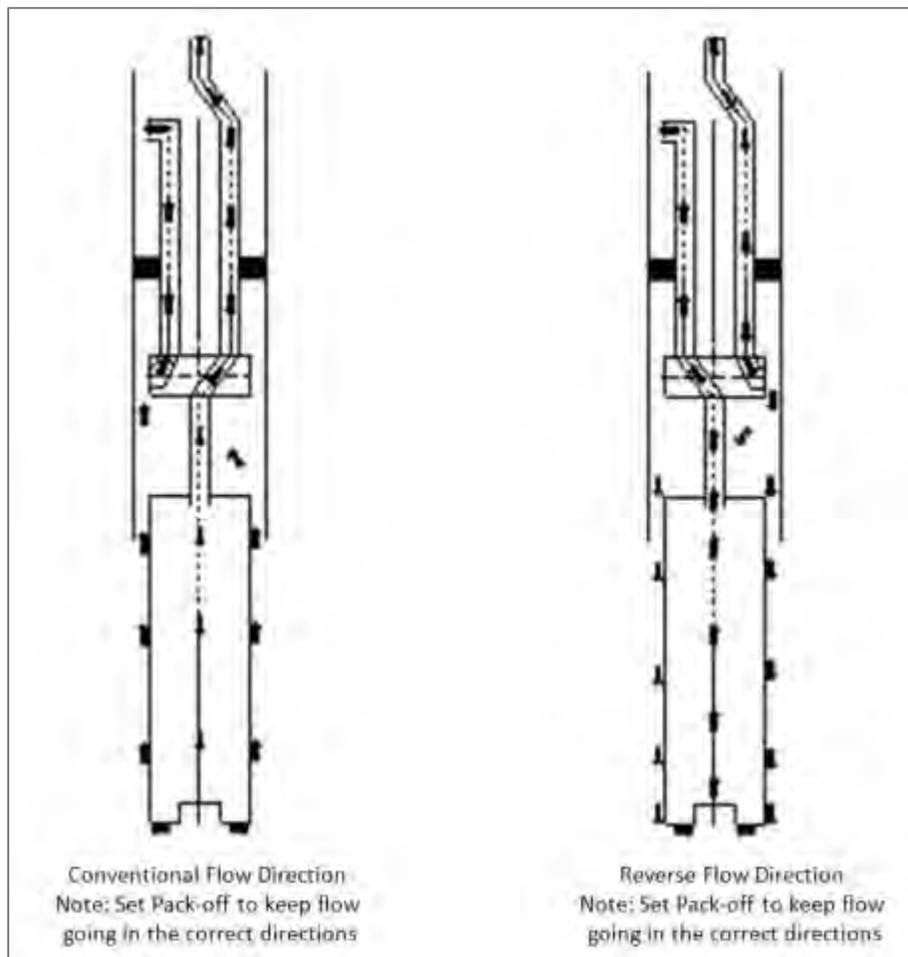
**Figure 3: Switchable crossover is run at the top of the casing**
