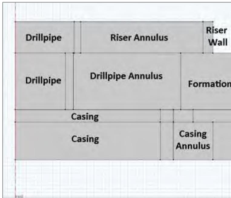
Figure 4. Simplified well geometry for FEA
