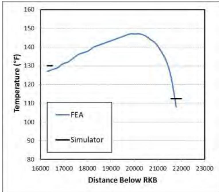
Figure 6. Temperature in the Cement and the end of the placement process
