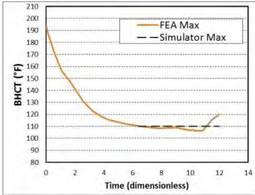
Figure 5. BHCT comparison between the FEA model and the simulator.
