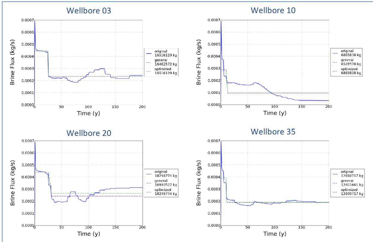
**Figure 4: Randomly selected brine input curves from numerical situations converted into a non- optimized and optimized general form input curve using Equation 4.**
