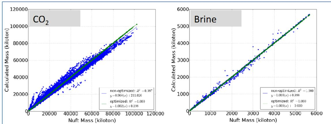
**Figure 5: Comparison of cumulative CO<sub>2</sub> (left) and brine (right) mass computed from the numerical models and generalized models. Each graph compares 48,000 data points based on non-optimized mass (blue dots) and optimized mass (green dots).**
