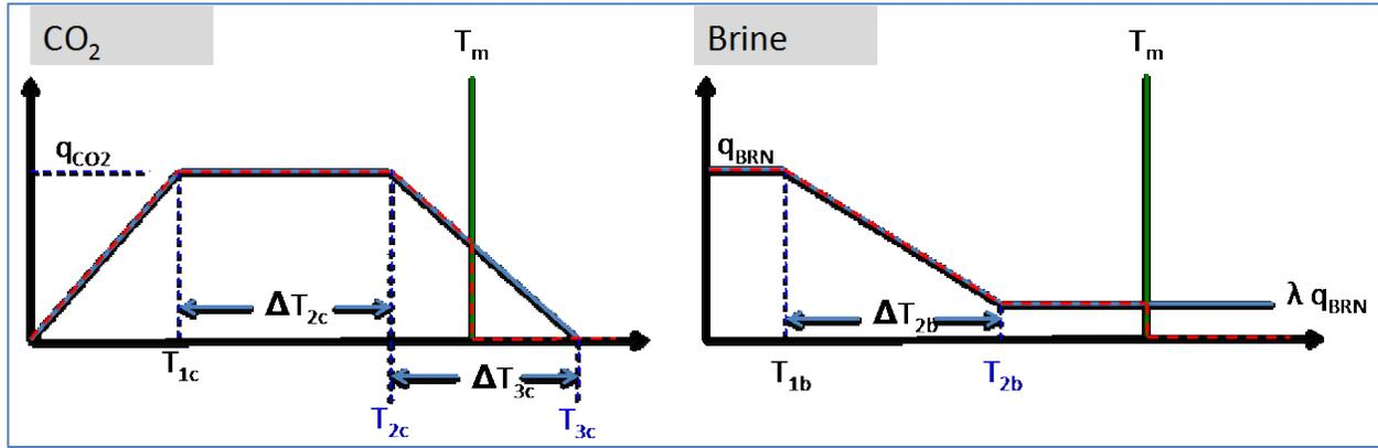
Figure 2: Basic shape of CO<sub>2</sub> (left) and brine (right) generalized input curves with parameters.
