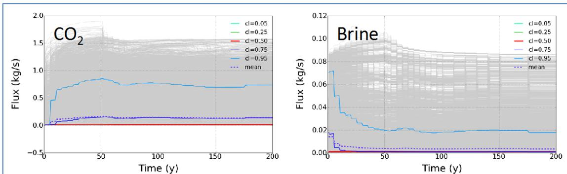
**Figure 1: CO<sub>2</sub> and brine fluxes resulting from numerical wellbore simulations with confidence intervals. Grey lines on each plot represent one of 48,000 flux curves.**
