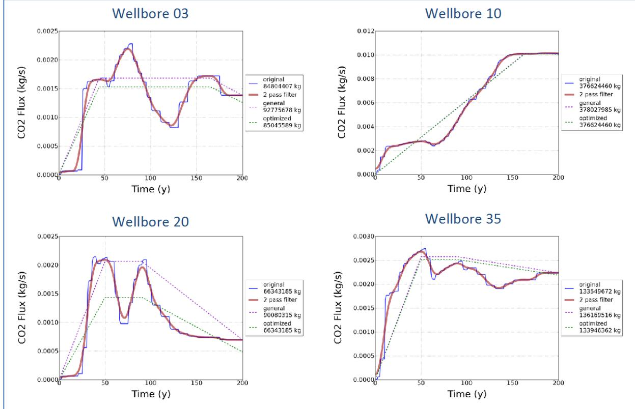
**Figure 3: Randomly selected CO<sub>2</sub> input curves from numerical situations converted into a non-optimized and optimized general form input function using Equation 2.**
