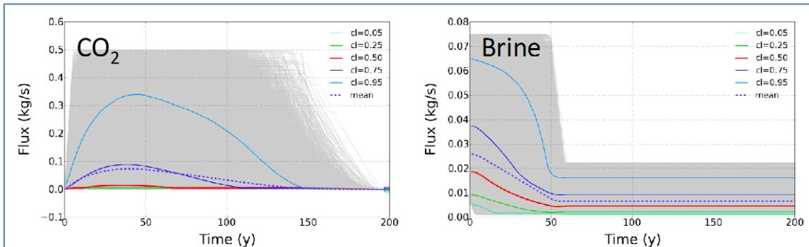
**Figure 6: Randomly generated CO<sub>2</sub> and brine fluxes for generalized model applying the parameter ranges listed in Table 1. Grey lines on each plot represent one of 48,000 flux curves. Mitigation time is omitted.**
