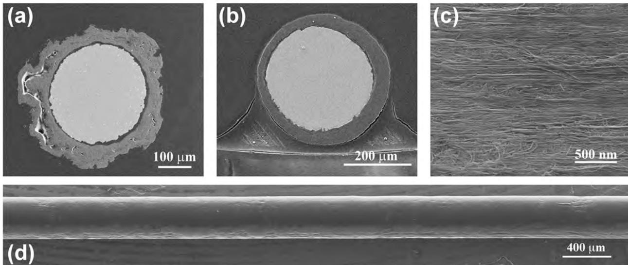
**Figure 3: SEM images of CNT coatings made from acid-based solutions. Images (a) and (b) are of a coated CNT wires with the sample in (b) having been wire drawn after coating. The SEM image (c) shows the relatively good CNT alignment within the coating. The long axis of the wire is parallel to the image bottom. The SEM composite image (d) shows an overall uniform surface morphology of a thick CNT coating after the wire drawing steps.**
