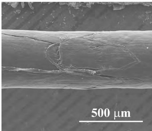
**Figure 4: SEM image of a crack structure in one of the CNT coated wires after wire drawing.**
