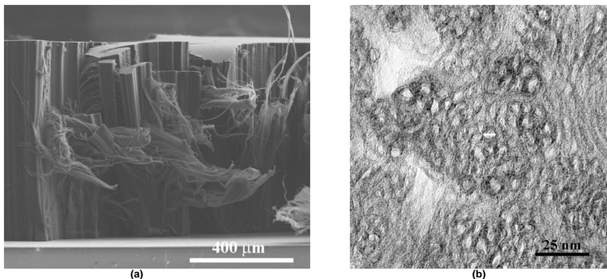
**Figure 1: SEM image (a) of an as-grown, 0.75 mm tall multi-wall CNT array that is the source for the CNT solutions in this work. TEM cross-sectional showing a cross-section of a CNT bundle. The white arrow in the center the cross-section of one CNT. The average diameter on the MW-CNTs was 10 nm.**
