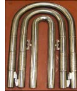
Cold bends and welds, B&W
