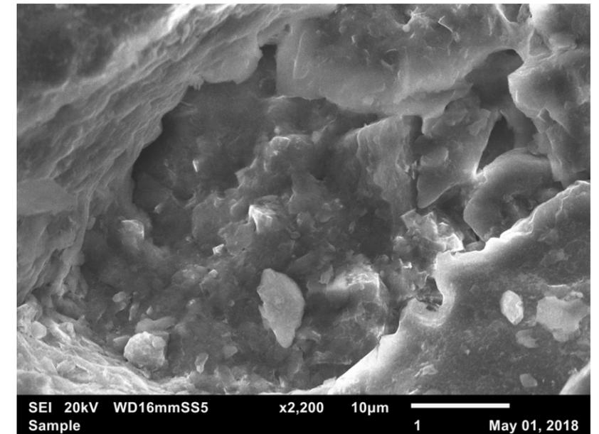
Figure 19: 20kV x2,200. Particles 1-10 micrometers in size are present.
