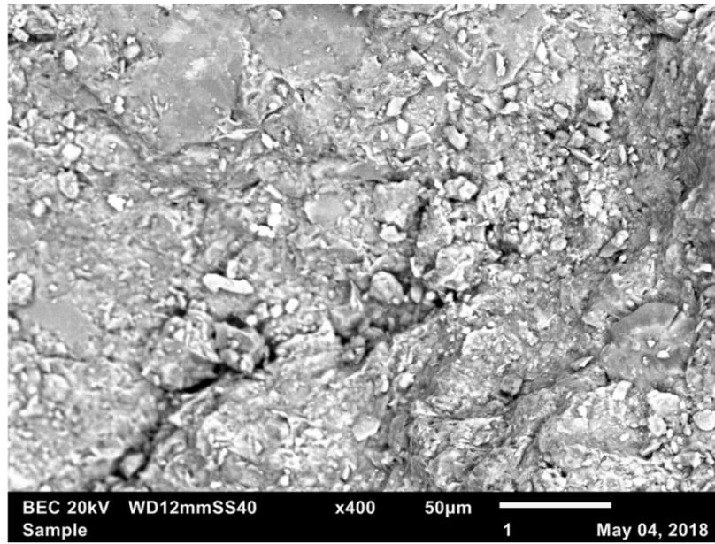
Figure 7: BEC 20kV x400. A variety of different sized particles make up the sample.
