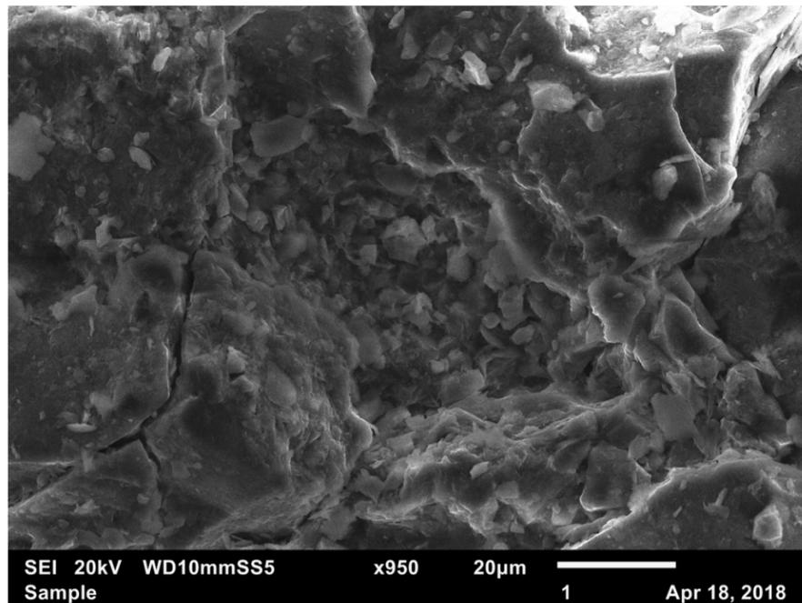
Figure 11: SEI 20kV x950. Most of the particles are flat, platy, and flaky. A crack in one of the grains is present in the bottom of this photomicrograph.
