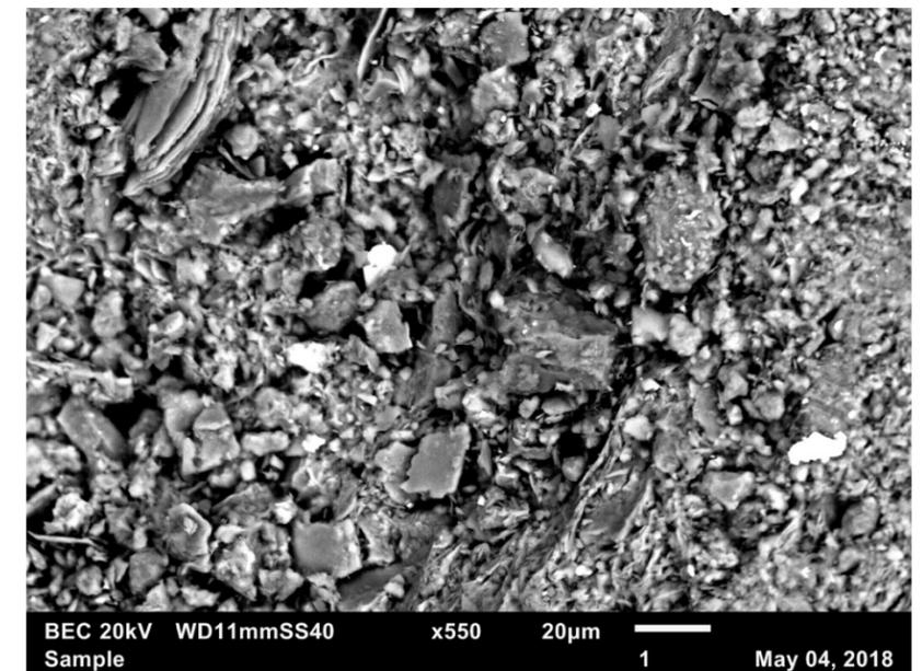
Figure 6: BEC 20kV x550. Corresponds to Figure 5. The gaps between some of the larger grains could be possible pore spaces.
