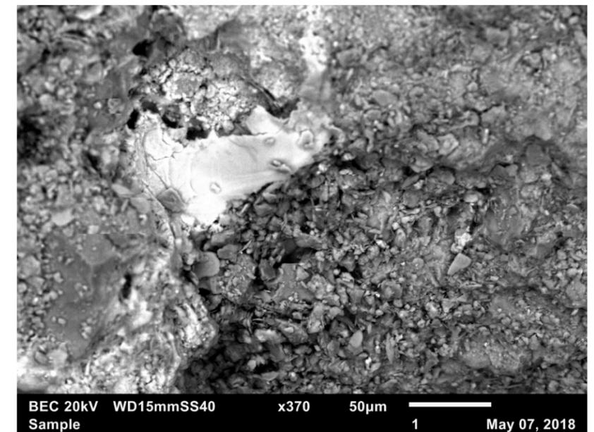
Figure 12: BEC 20kV x370. Corresponds to Figure 11. The larger mineral in Figure 11 is white in this photomicrograph. This indicates that the grain is of a different composition than its surrounding minerals.
