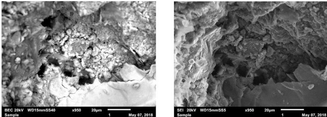
Figure 5: Observable porosity in the 2690-2700 ft interval of the Gordon sand. The darker the void space, the deeper the pore.
