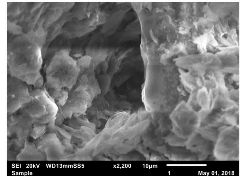
Figure 23: SEI 20kV x2,200. A closer look into the pore. The flat, platy minerals extend into the space.
