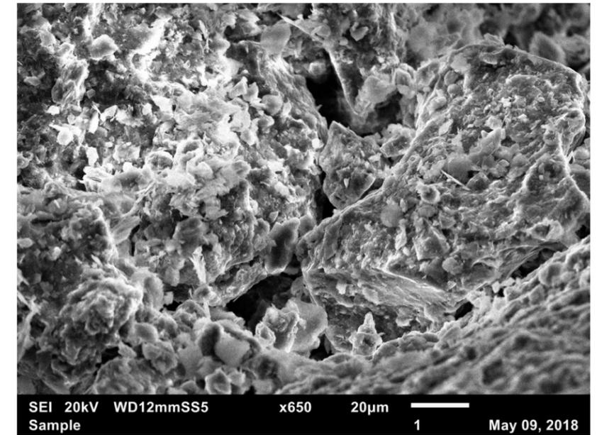
Figure 5: SEI 20kV x650. Pore space is observed around the 100-micrometer grain.
