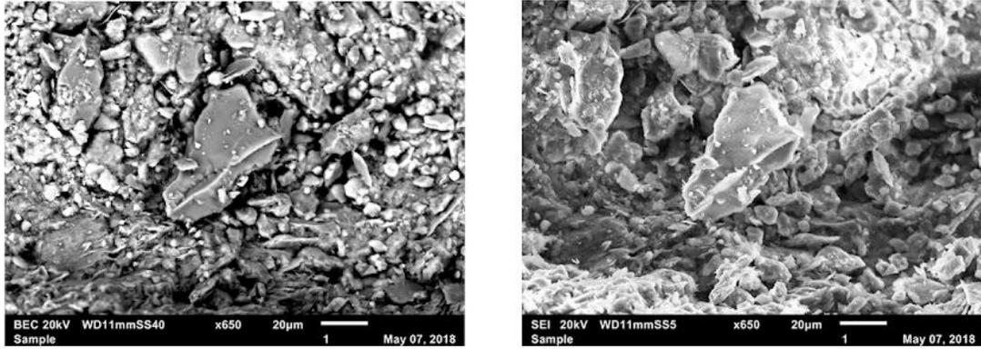
Figure 3: BEC and SEI pictures of the 2690-2700 ft interval of the Gordon sand. The contrasting images give insight into the chemical makeup of this sample, which appears to be mostly clay.
