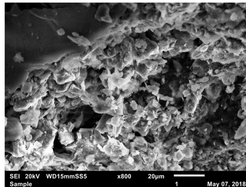
Figure 16: SEI 20kV x800. Platy clay minerals and possible porosity are shown.
