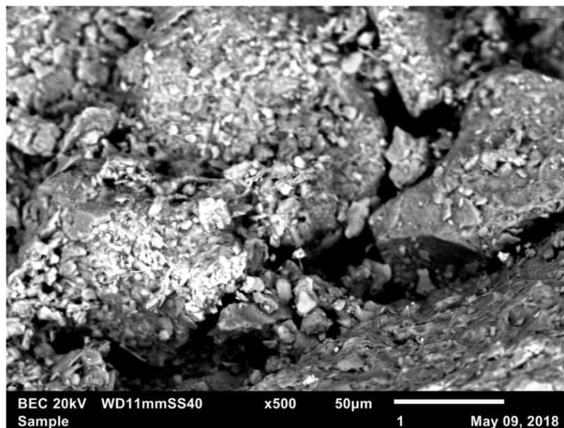
Figure 14: BEC 20kV x500. Corresponds to Figure 13. Pore space is observed between the larger grains.
