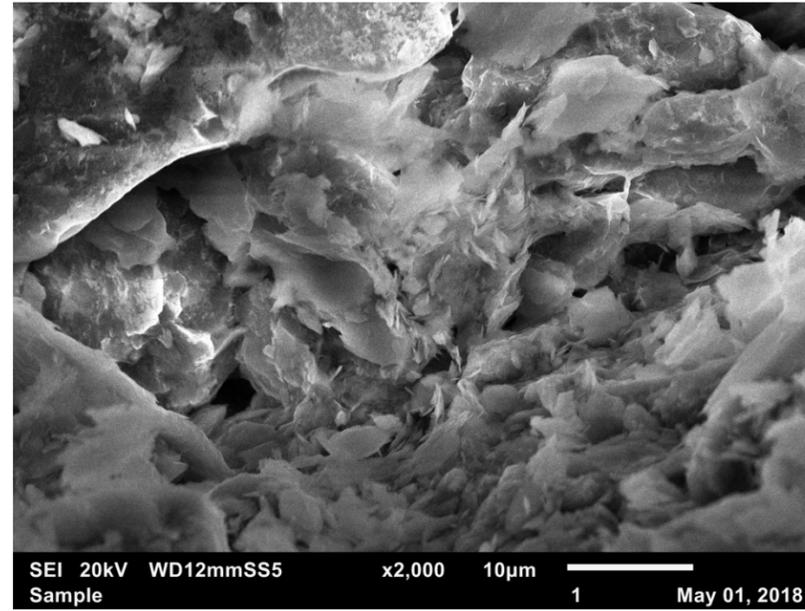
Figure 26: SEI 20kV x2,000. A closer look at the minerals in Figures 24 and 25. Some porosity may be present—a few gaps around 2-3 micrometers in diameter can be seen in the center of the photomicrograph.
