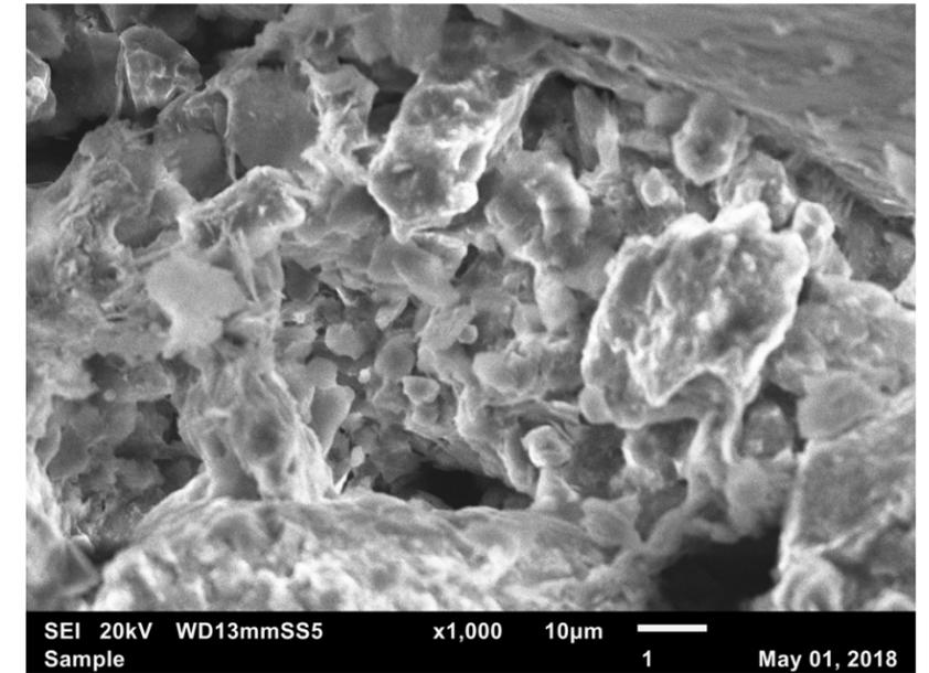
Figure 28: SEI 20kV x1000. Corresponds to Figure 27. A closer look at the gaps of this section as well as the flat, platy minerals composing the sample
