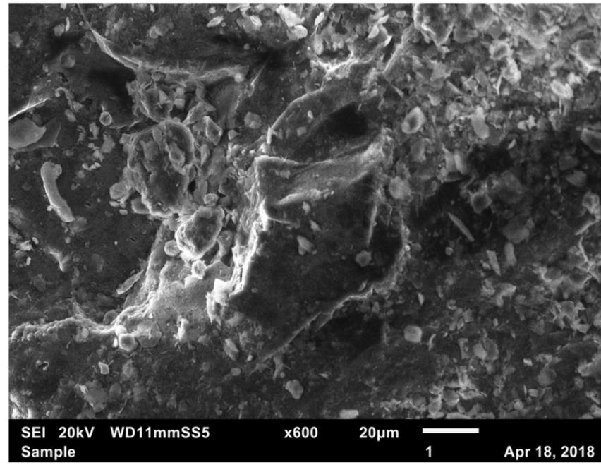
Figure 12: SEI 20kV x600. Smaller silt to clay-sized particles coat the surface of the sample.
