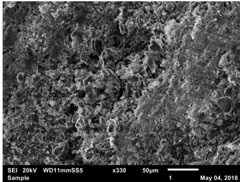
Figure 1: SEI 20kV x330. Flat, platy particles ranging 10-50 micrometers in diameter make up the surface of this sample.
