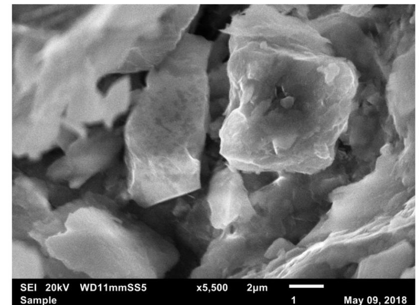
Figure 18: SEI 20kV x5,500. Corresponds to the upper center portion of Figure 17. The mineral pictured is cubic in shape, and the texture appears to be flaky and platy.
