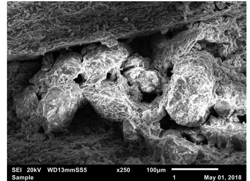
Figure 4: SEI 2kV x250. Large pores are visible between these grains. Large particles over 100 micrometers in diameter and smaller particles less than 10 micrometers are present.
