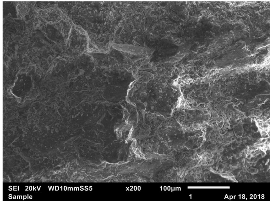
Figure 5: SEI 20kV x200. Platy clay minerals on the surface of the sample.
