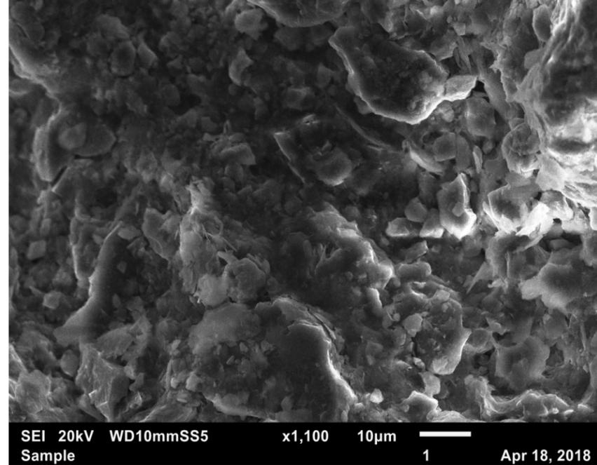
Figure 13: SEI 20kV x1,100. The particles are rounded to sub-rounded.
