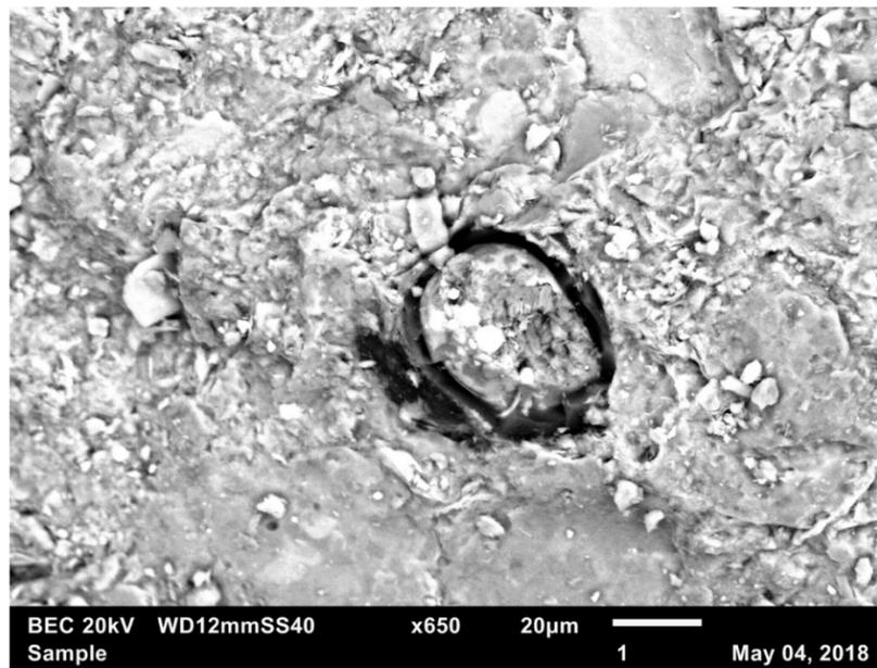
Figure 8: BEC 20kV x650. A grain around 40 micrometers across is surrounded by a gap.
