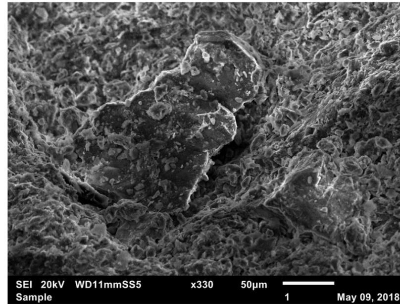
Figure 3: SEI 20kV x330. A large grain around 200 micrometers across is surrounded by particles 10 micrometers in diameter.
