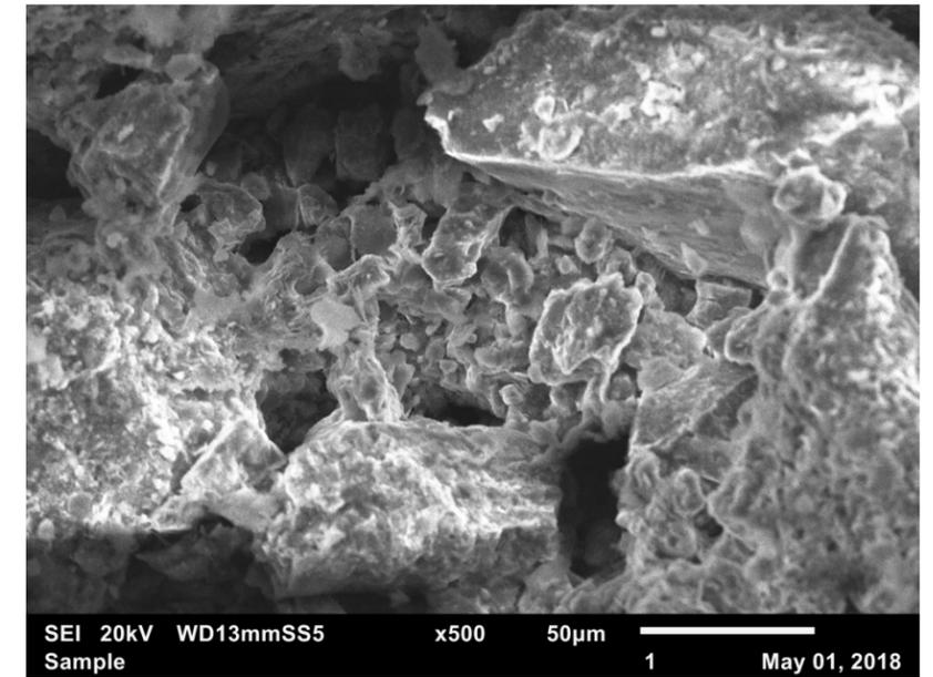
Figure 27: SEI 20kV x500. The gaps present may be instances of porosity.
