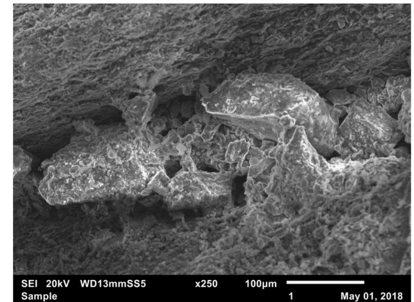
Figure 15: SEI 20kV x250. Some porosity present between the largest grains.
