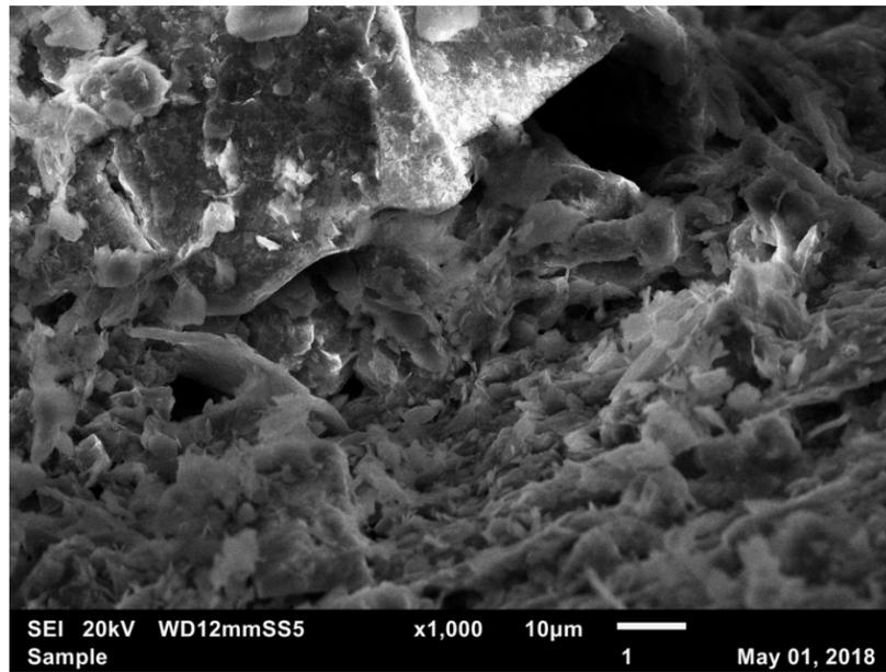
Figure 25: SEI 20kV x1,000. Corresponds to Figure 24—a closer look at the “gaps”. What appeared to be a possible pore in Figure 24 was just a dark spot in the photomicrograph. Platy minerals can be seen in a higher magnification.
