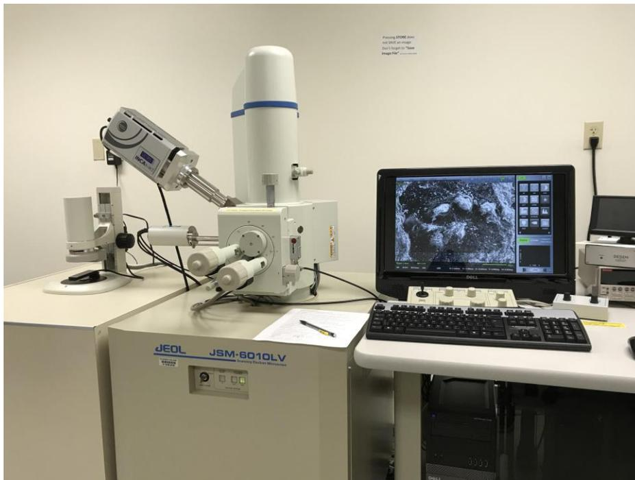
Figure 1: The SEM machine alongside the monitor used to view the images.
