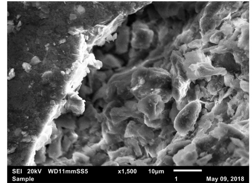
Figure 17: SEI 20kV x1,500. Details of the smaller particles of the sample. The platy and flaky minerals range from 1 to 10 micrometers in diameter.
