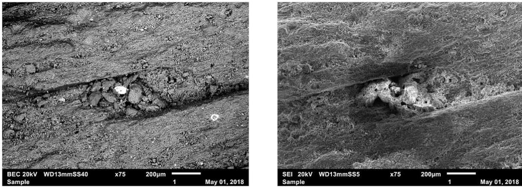
Figure 4: BEC and SEI pictures of the 2672-2680 ft interval of the Gordon sand. The white mineral in the BEC image may be an oxide or sulfide such as pyrite or magnesite.
