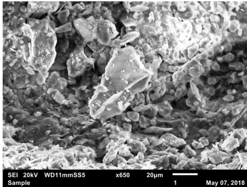
Figure 7: SEI 20kV x650. Particles of varying sizes ranging from 50 to 5 micrometers across make up the sample.
