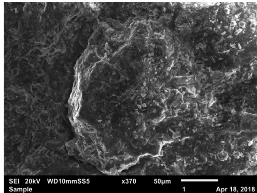
Figure 8: SEI 20kV x370. A larger grain surrounded by clay minerals.
