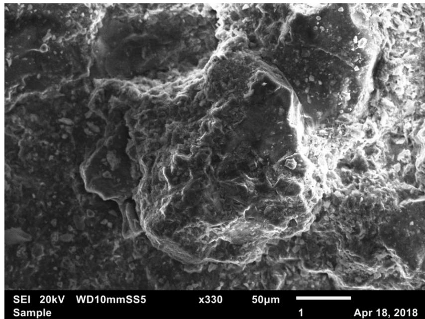
Figure 6: SEI 20kV x330. Platy clay particles surrounding larger fine sand or coarse silt grains.
