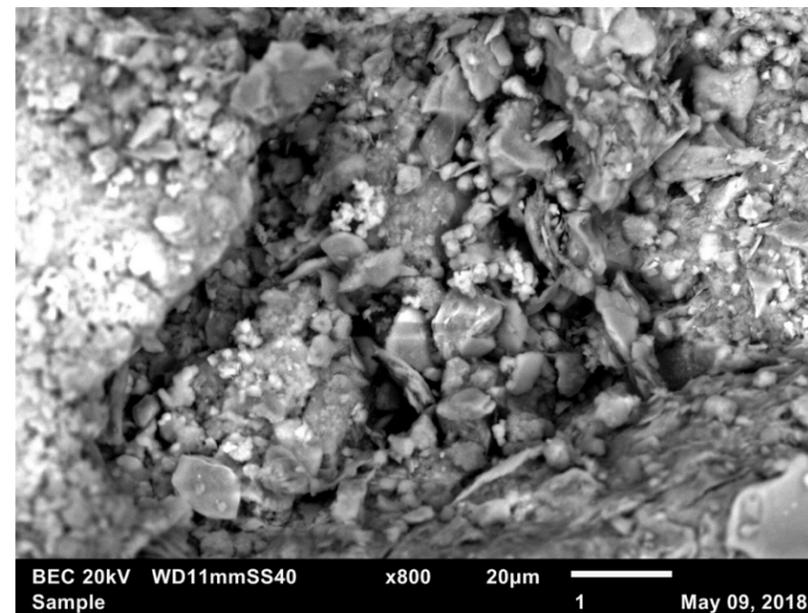
Figure 10: BEC 20kV x800. Corresponds to Figure 9. The BEC photomicrograph of this section shows that what looked like possible pore space in the sample was just a dark spot in the picture.
