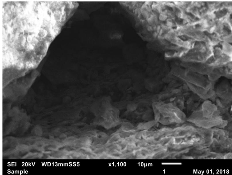
Figure 7: SEI 20kV x1,100. An even closer look at the same pore from Figure 4. Platy particles 10 micrometers or less can be seen coating the larger grains.
