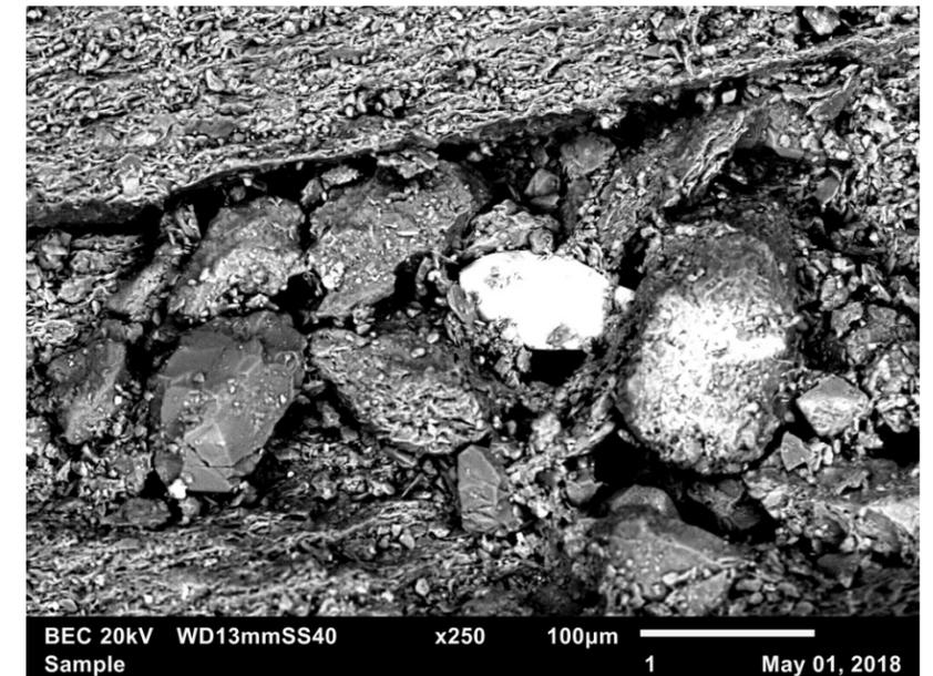
Figure 5: BEC, 20kV x250. Observable porosity in the sample. The white-appearing grain is most likely an oxide or sulfide.
