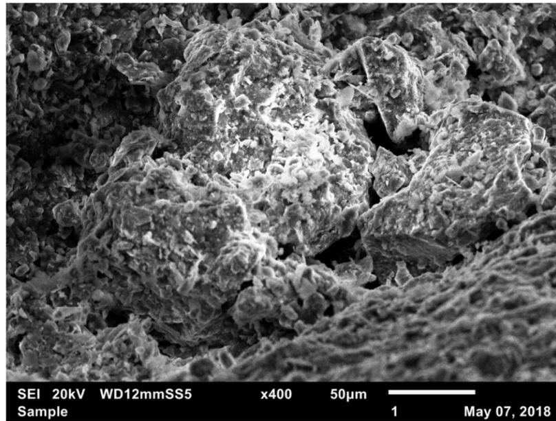
Figure 13: SEI 20kV x400. Larger grains around 100 micrometers in diameter are center in this section. Possible pore space lies in between the large grains.
