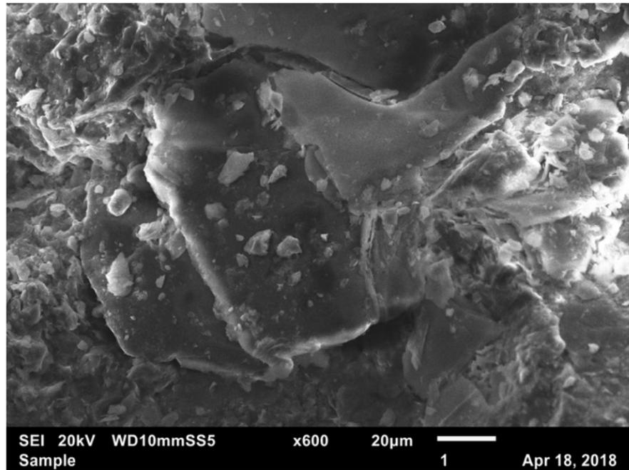
Figure 10: SEI 20kV x600. Particle size ranges from micrometers to 100 micrometers.
