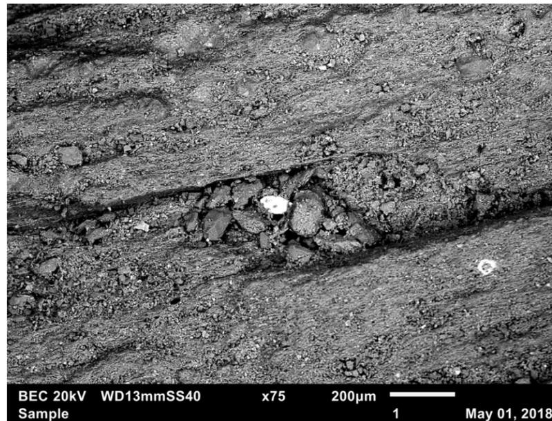
Figure 3: BEC 20 kV x75. The BEC image displays the differing composition of the grains.
