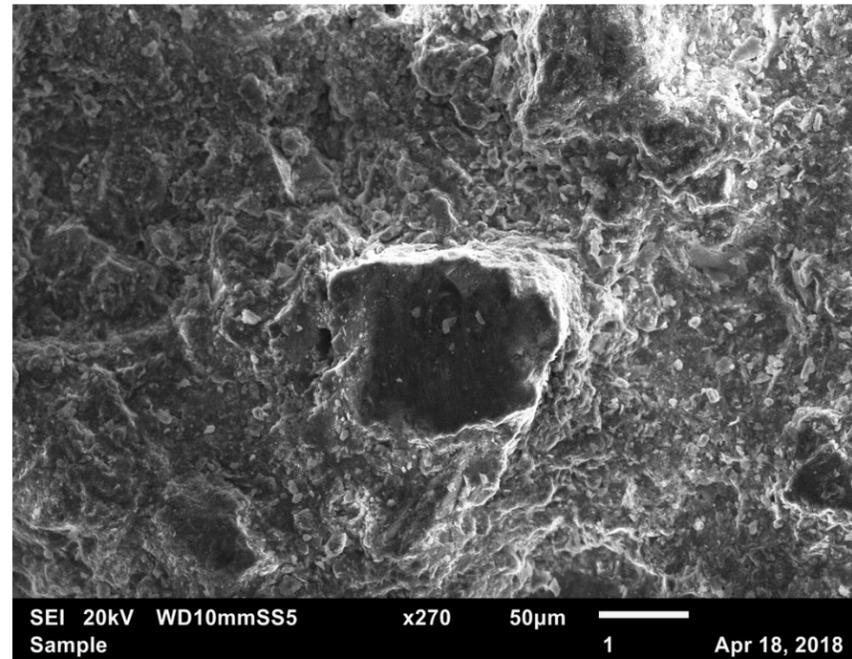
Figure 7: SEI 20kV x270. A larger particle surrounded by clay minerals.
