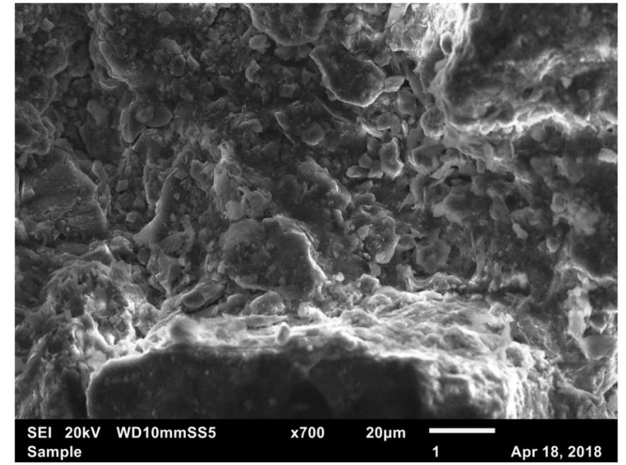
Figure 14: SEI 20kV x700. Very fine silt and clay particles lie on top of and between larger coarse silt particles, serving as the cement of the rock.
