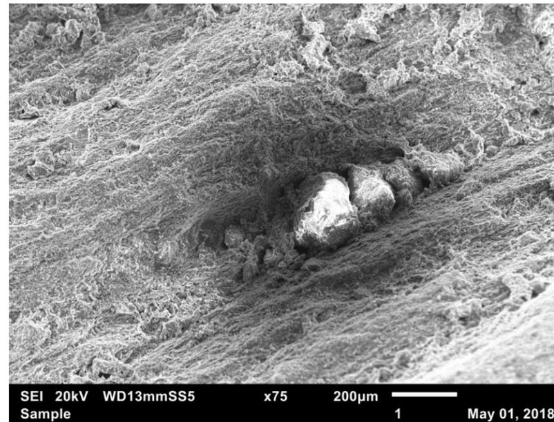
Figure 9: SEI 20kV x75. A closer look at the grains in Figure 8. A 200-micrometer grain is present in the center of the photomicrograph. No observable porosity.
