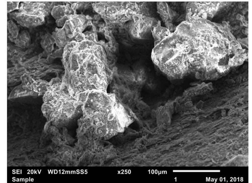
Figure 11: SEI 20kV x250. A closer look at Figure 10. Possible porosity between the larger grains.
