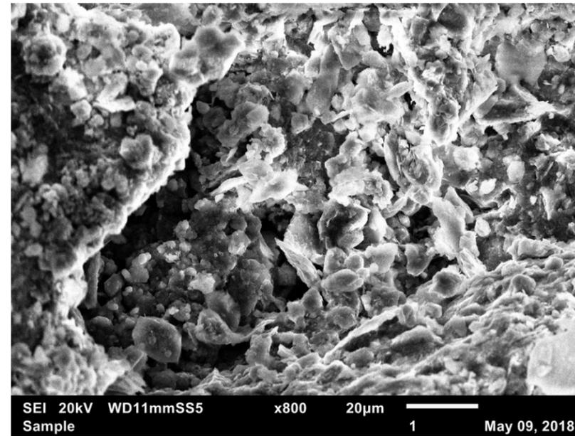
Figure 9: SEI 20kV x800. Pore space seems to be present towards the left of the sample are.
