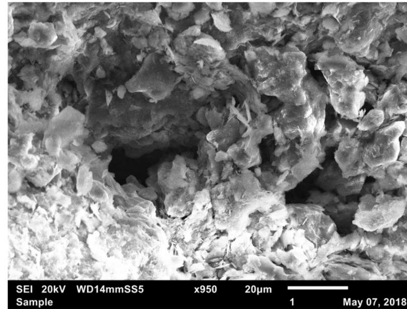
Figure 15: SEI 20kV x950. Porosity as well as flaky minerals are present in this sample.
