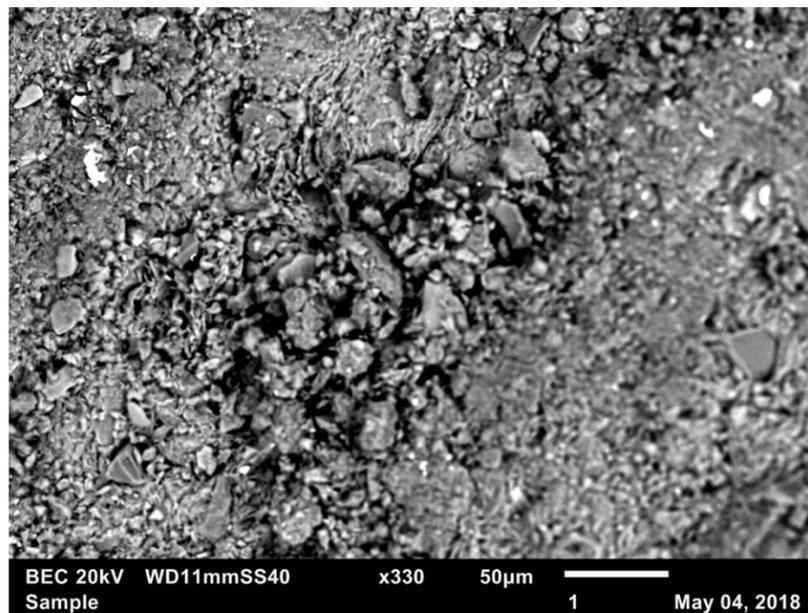
Figure 2: BEC 20kV x330. Corresponds to Figure 1. There could be some pore space between the grains larger than 25 micrometers in the center of the sample.
