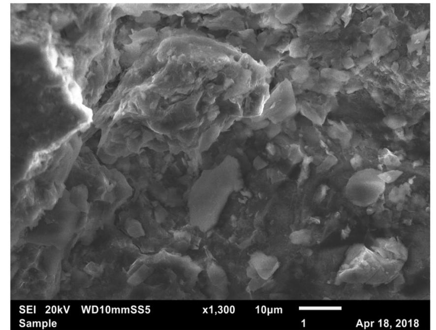
Figure 15: SEI 20kV x1,300. Clay-size particles 1 micrometer in diameter are present.
