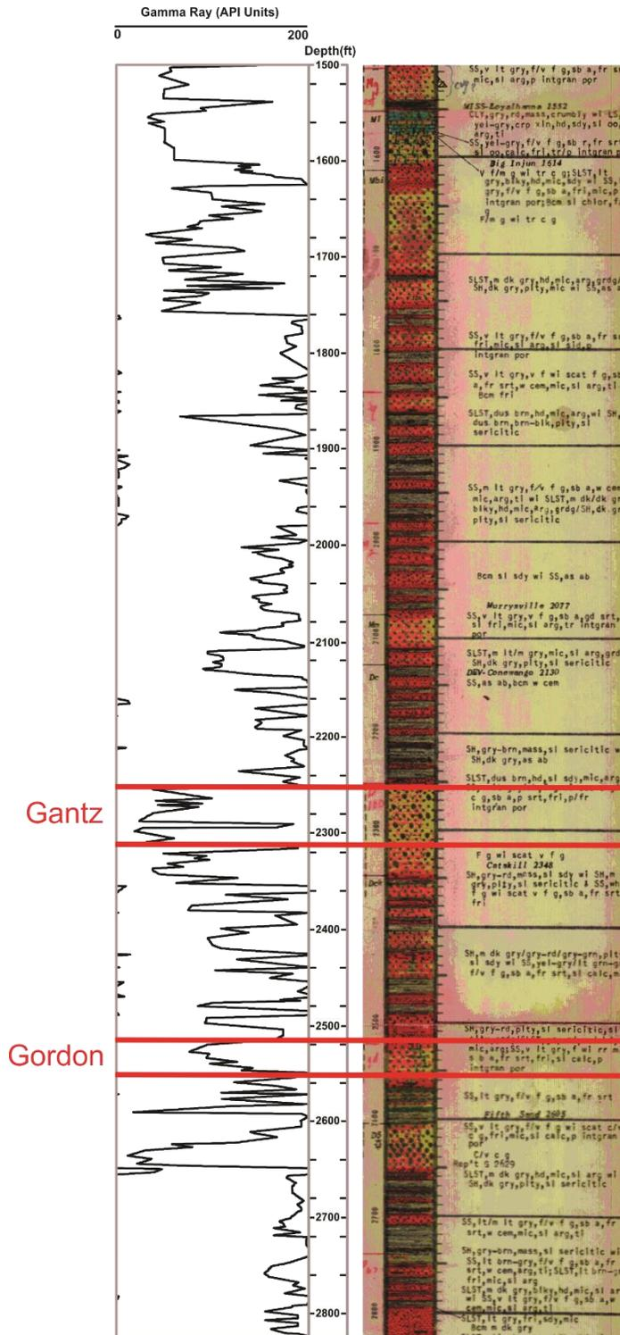
Figure 6: Geophysical logs of the #3299 Hamilton well. The GR curve is on the left and the GEO log is on the right. The Gantz and Gordon sandstone intervals are marked.
