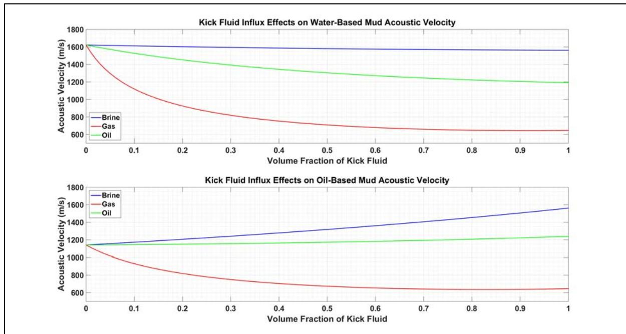
**Figure 4: Effects of kick fluid mixing on drilling fluid acoustic/sonic velocity.**
