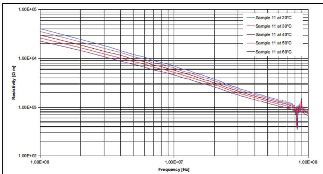
Figure 2: Temperature effect on resistivity – Sample 11 (Patil et al., 2010).
