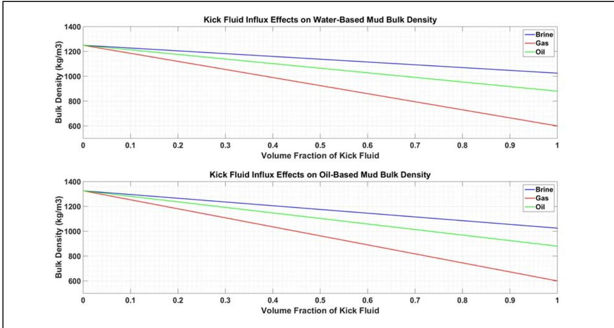
Figure 1: Effects of kick fluid mixing on drilling fluid bulk density.
