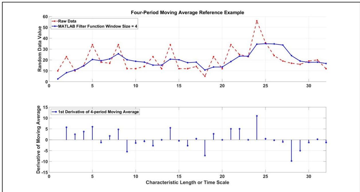
**Figure 6: Moving average differential for kick identification.**
