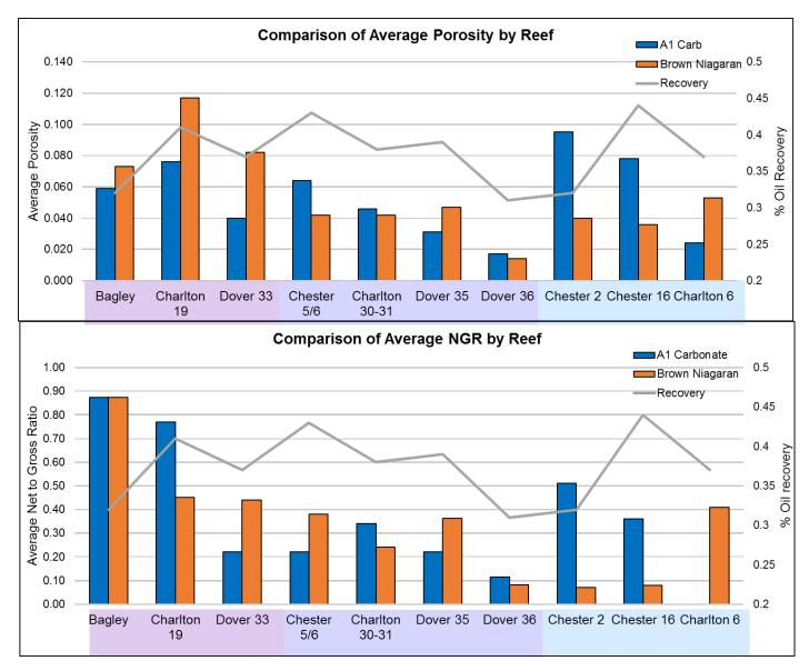
Figure 16-2. Comparison of average porosity, NTG ratio, and percent recovery by reef. Along the horizontal axis, light purple shading (left) = dolomitic, light blue shading (right) = limestone, and lavender (center) = mixed carbonate.
