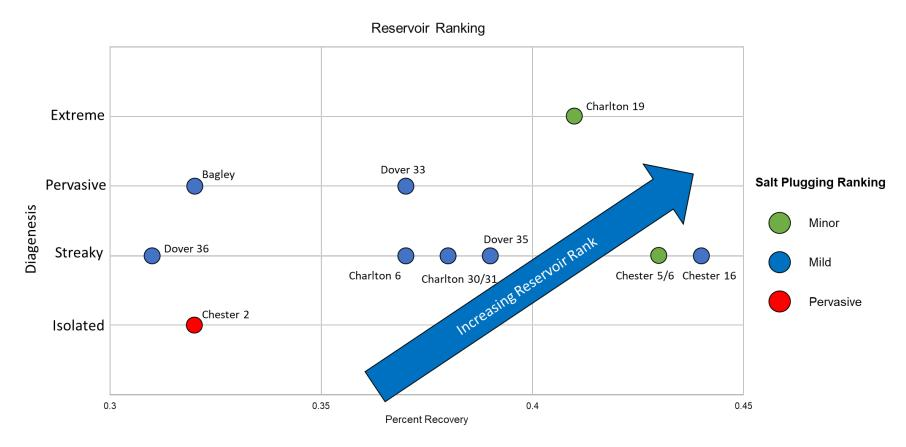
Figure 16-4. Reservoir ranking plot of reefs using diagenesis and salt plugging rank with percent oil recovery.
