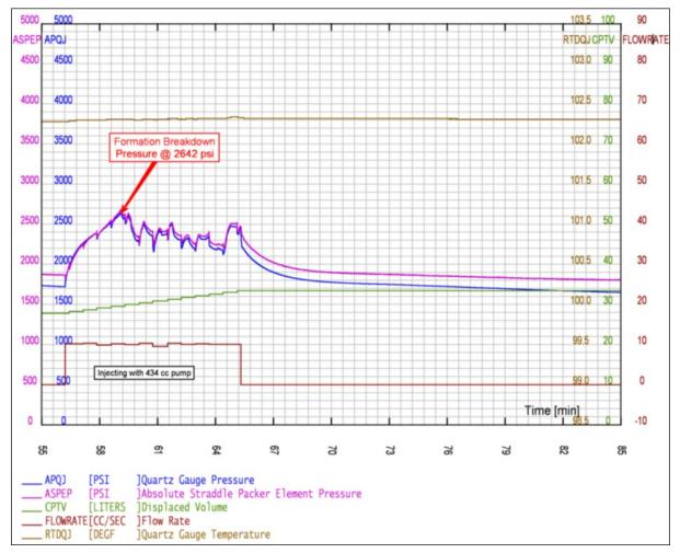
Figure 4-13. Fracture Breakdown Pressure During the First Injection Cycle (FOT1) of MicroFrac Test 1.
