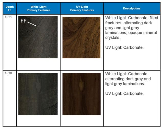
Figure 2-14. Annotated RSWC images with corresponding core descriptions of the A-2 Carbonate for depths 5,761 ft. and 5,778 ft.
