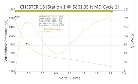
Figure 15-58. Example G-function of shut-in time plot for fracture closure identification in station 1/cycle 1.
