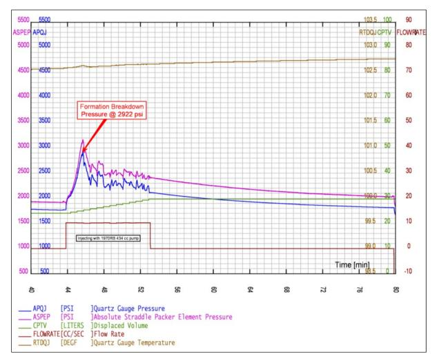
Figure 15-60. Fracture breakdown pressure during the FOT1 of micro-frac test 2.
