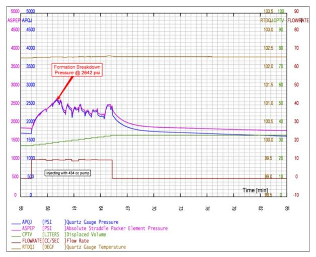
Figure 15-55. Fracture breakdown pressure during FOT1 of micro-frac test 1.
