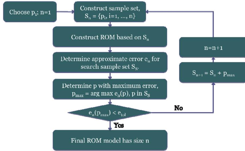
Figure 1: Flow diagram for the adaptive sampling procedure.  $S_n$  is the sample set evaluated by the high-fidelity model to build the ROM,  $S_S$  is a set of potential sampling points in which to search for the parameter point with the largest estimated approximation error.
