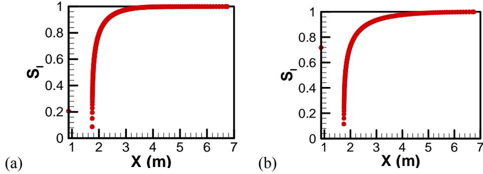
Figure 2: Liquid saturation at (a) 10 days; and (b) 40 days for  $\log(k)=-15$ ,  $n=2$  and  $\log(1/\alpha)=6$ .  $X$  is the radial distance to the tunnel. The first data point (red dot) shows the liquid saturation of the tunnel element. Interested model output is at  $X=1.77$  m, 2cm away from the tunnel.
