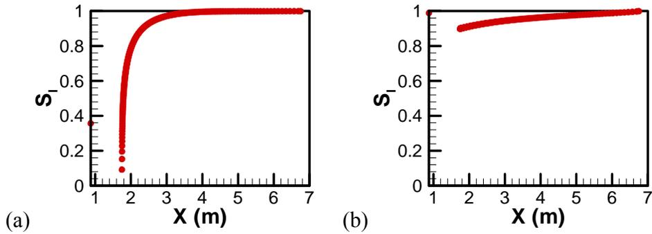
Figure 3: Liquid saturation at (a) 10 days; and (b) 40 days for  $\log(k)=-14.75$ ,  $n=2$  and  $\log(1/\alpha)=6$ .  $X$  is the radial distance to the tunnel. The first data point (red dot) shows the liquid saturation of the tunnel element. Interested model output is at  $X=1.77$  m, 2cm away from the tunnel.
