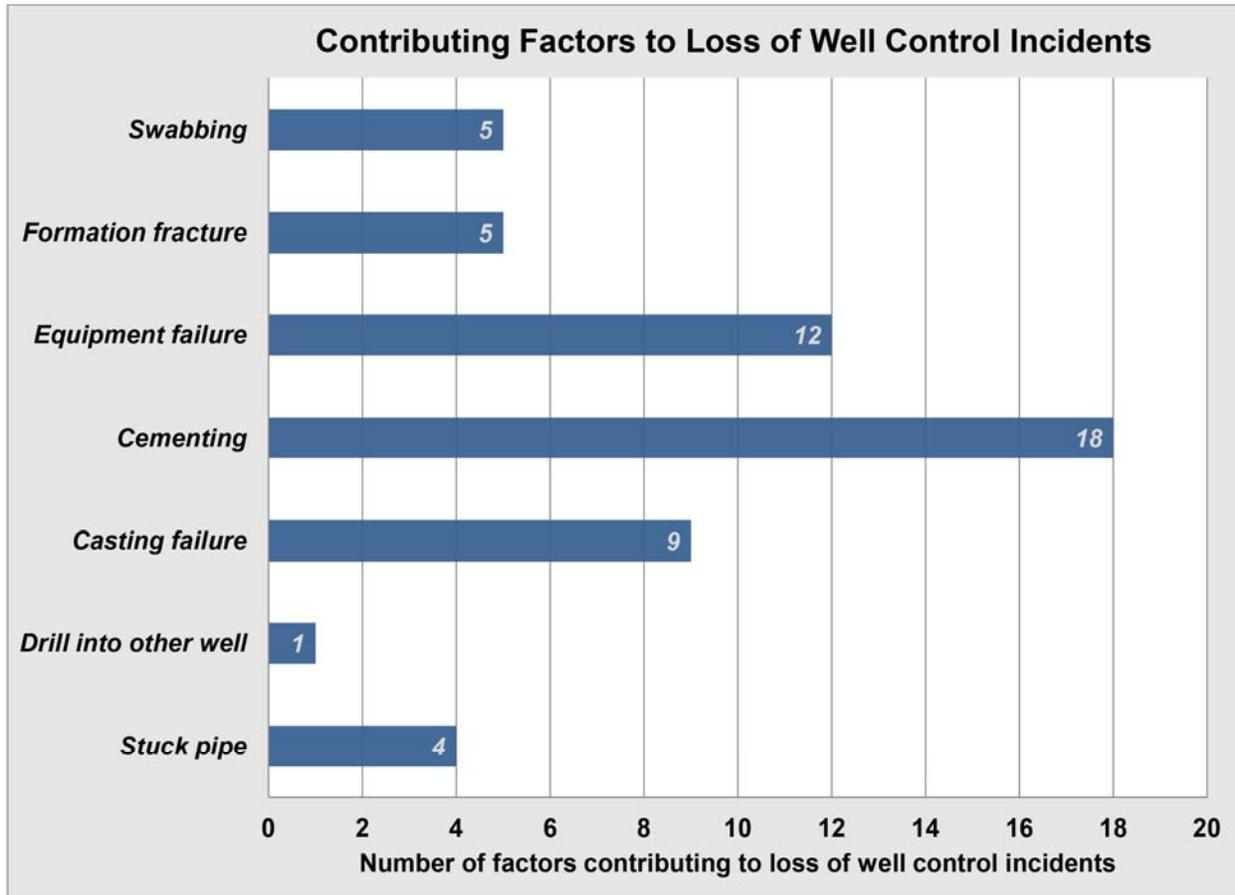
**Figure 1: Data from offshore operations in the Gulf of Mexico spanning 1992 to 2006 clearly demonstrates the significant role cement barriers play in ensuring safe and productive operations during the drilling and completion phase of a well (Izon et al., 2007).**
