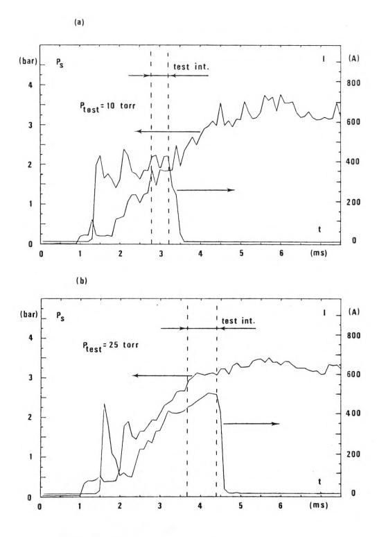
Fig. 2. a) Stagnation pressure  $(P_s)$  and Hall current (I) history for a low pressure of the test gas  $(P_{test})$  prior to the rupture of the shock tube diafragmes. The test interval is also indicated.
