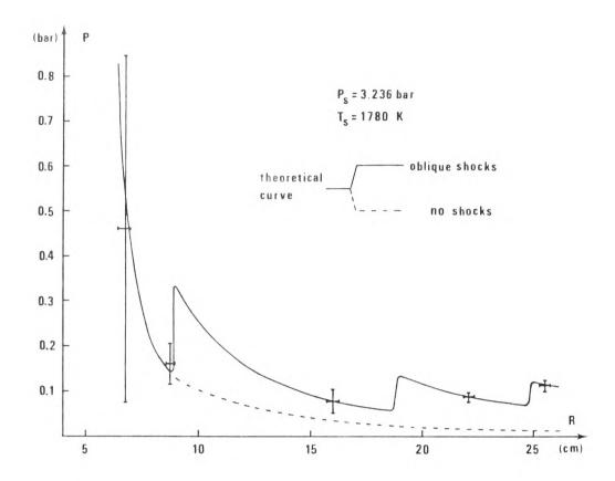
Fig. 3. Calculated radial profile of the static pressure P and experimental values (with their errors) for zero magnetic interaction. The entrance stagnation pressure  $P_s$  and stagnation temperature  $T_s$  are indicated.
