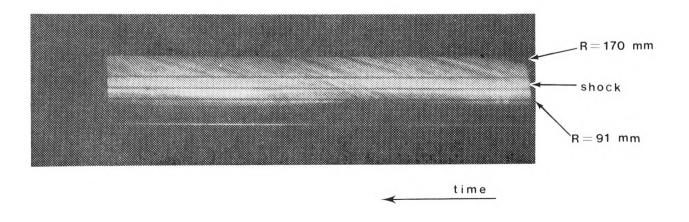
Fig. 4. Streak photograph of the radial disk generator at conditions of considerable magnetic interaction:  $P_{_{\rm S}} = 3.05~{\rm bar},~T_{_{\rm S}} = 2090~{\rm K},~B = 1.8~{\rm T},$
