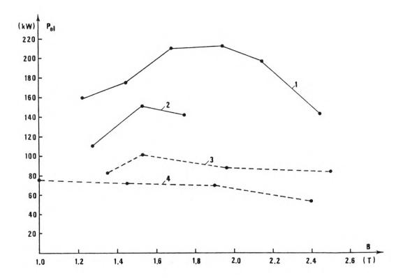
Fig. 5. Output power ( $P_{el}$ ) versus magnetic induction (B). Curves 1,2: load connected between  $A_2$  and C; curves3,4: load connected between  $A_1$  and C ( $A_1$ ,  $A_2$ , C - see fig.1.a). The operating conditions are: curve 1 seed fraction 0.02 % |  $P_s$ =2.9 bar,  $T_s$ =2130 K, curve 2 seed fraction 0.045 % |  $P_s$ =0.19 Ohm curve 3 seed fraction 0.08 % |  $P_s$ =2.15 bar,  $T_s$ =2600 K, curve 4 seed fraction 0.2 % |  $P_s$ =0.50 Ohm
