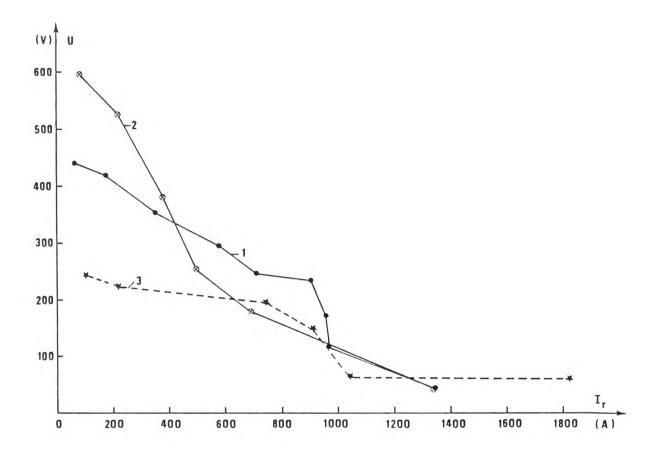
Fig. 6. Voltage to current characteristics of the generator. Curves 1,2: load connected between  $A_2$  and C; curve 3: load connected between  $A_1$  and C ( $A_1$ ,  $A_2$ , C - see fig. 1,a). The operating conditions are: curve 1  $P_s$ =3.0 bar,  $T_s$ =2100 K, B=1.75 T, seed fraction 0.03 % curve 2  $P_s$ =3.35 bar,  $T_s$ =1870 K, B=2.85 T, seed fraction 0.008 % curve 3  $P_s$ =2.2 bar,  $T_s$ =2600 K, B=1.30 T, seed fraction 0.04 %
