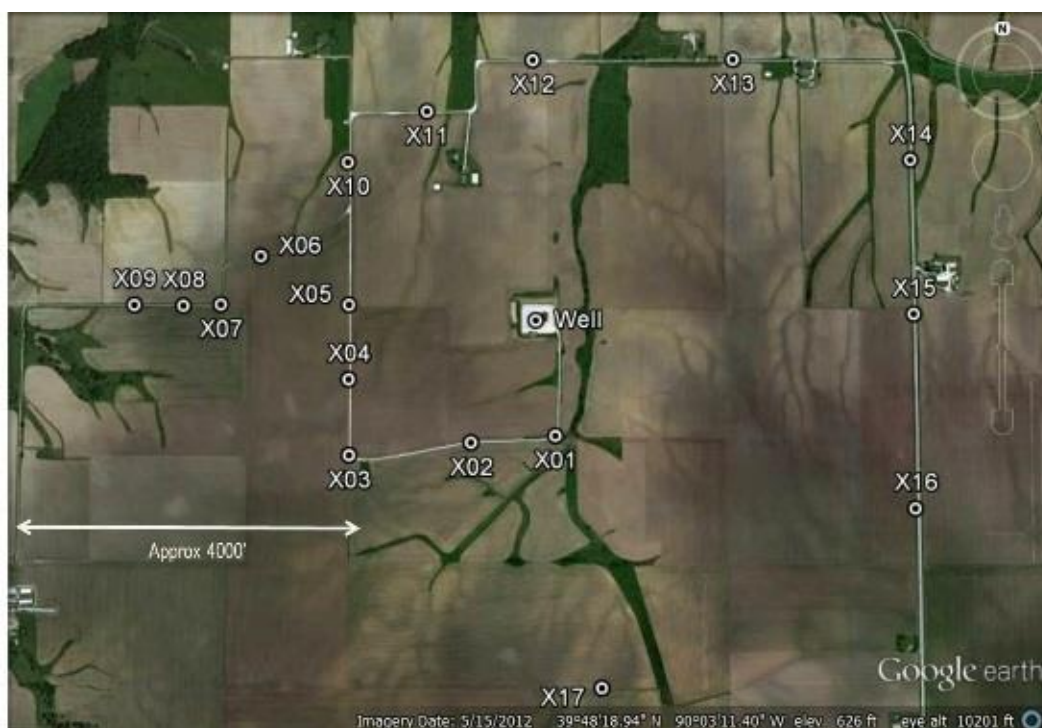
Figure 3-2. Map showing locations of VSP source stations around the FutureGen2 VSP receiver well.
