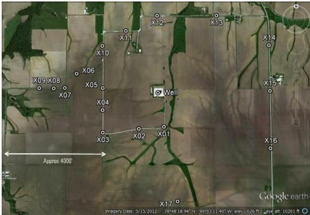
Figure 1-2. VSP well and source locations X01 through X17 at the FutureGen2 site. No data were generated at source stations X04 and X06.
