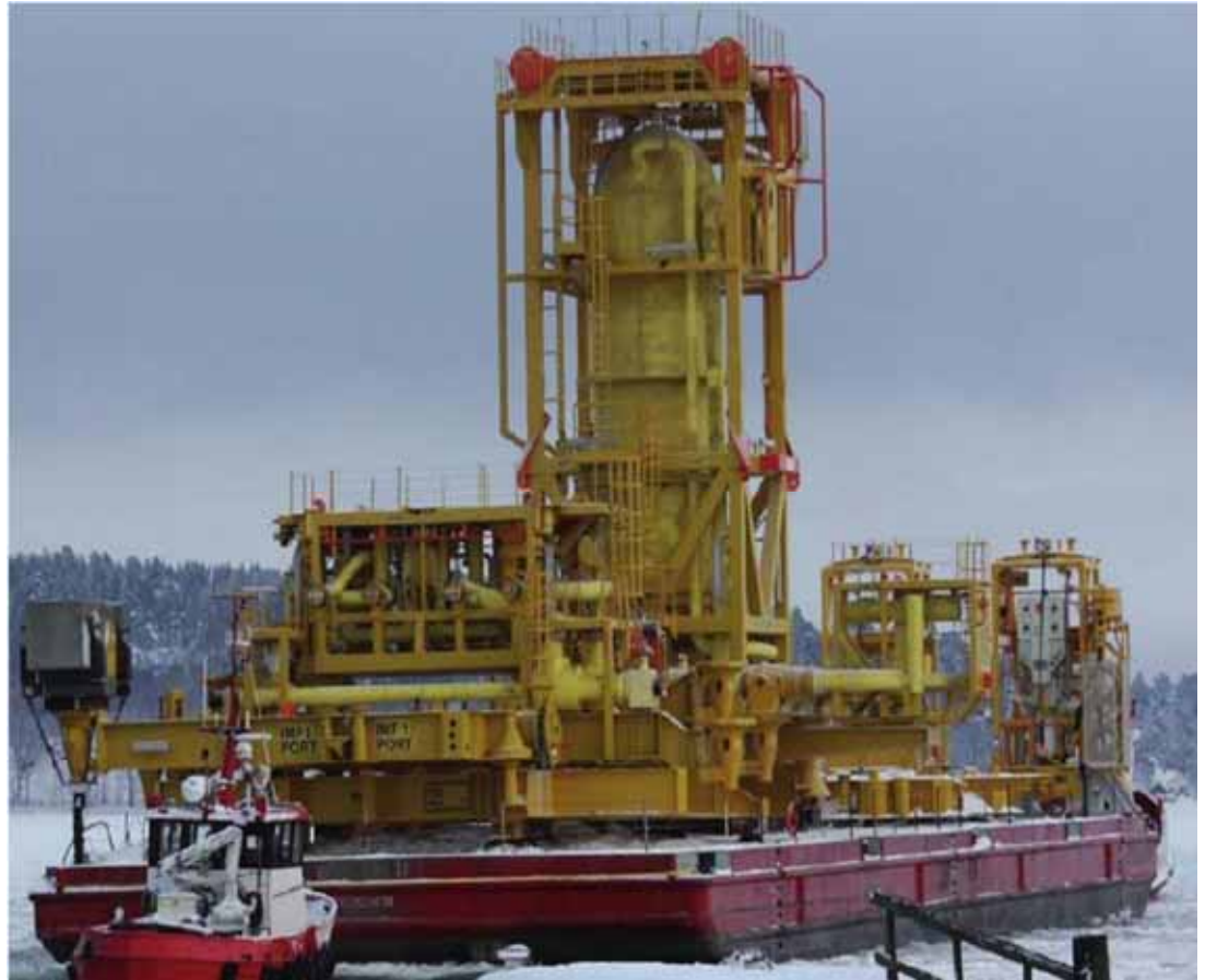
FMC Pazflor SS Gas/Liquid Separation & Boosting, Courtesy of FMC
