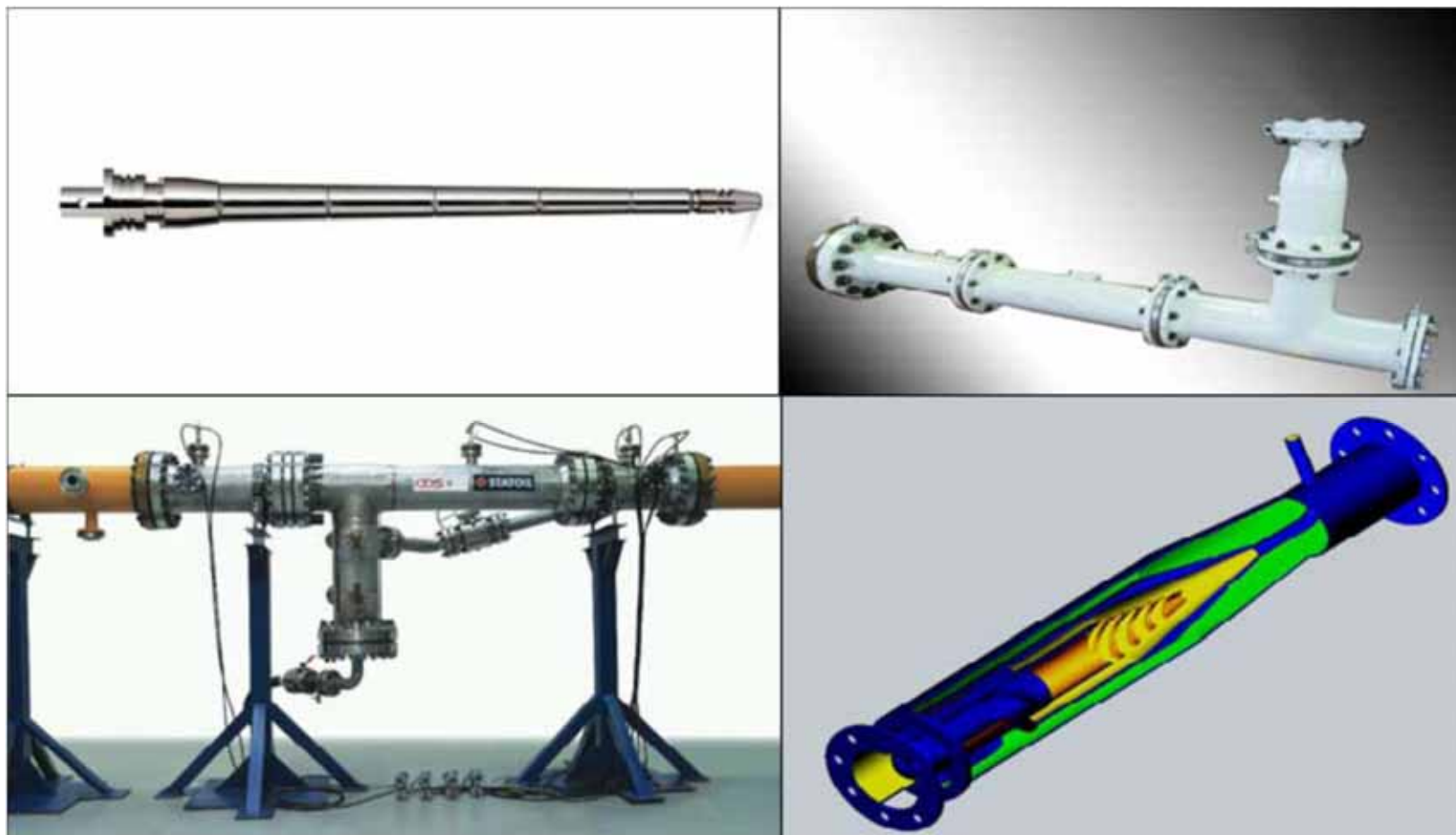
Inline Cyclonic Separation Equipment - Clockwise: Liquid-Liquid Separation, Phase Splitter, De-Sander, Deliquidizer, (Courtesy of OTC 20080 paper, 2009)
