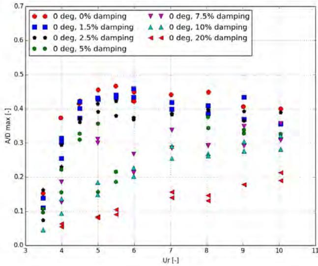
Figure 10: Paired-column semi maximum cross-flow amplitudes for 0 degrees heading
