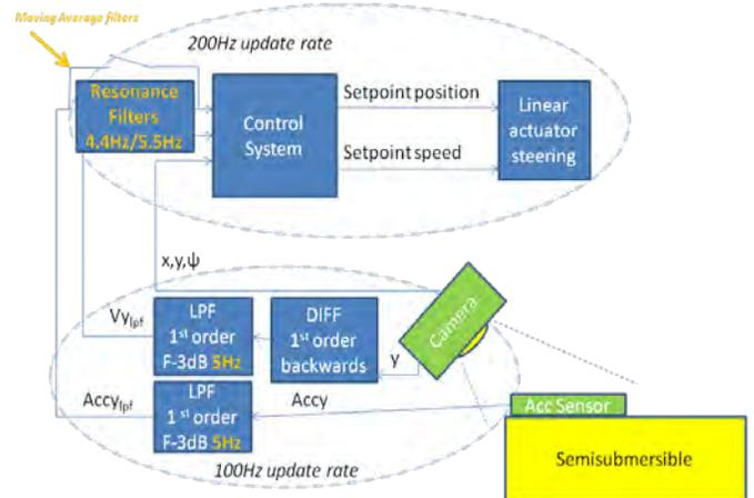
Figure 7: Overview working principle active damping system
