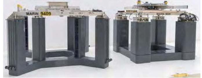
**Figure 1: Paired column semi (left) and four column semi model**
