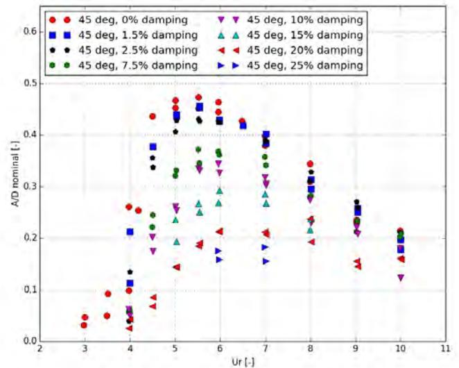
Figure 13: Four column semi nominal cross-flow amplitudes for 45 degrees heading
