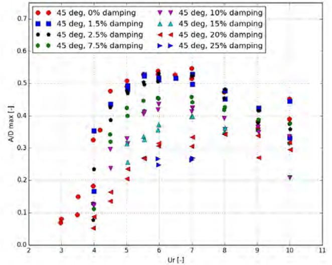
Figure 12: Four column semi maximum cross-flow amplitudes for 45 degrees heading
