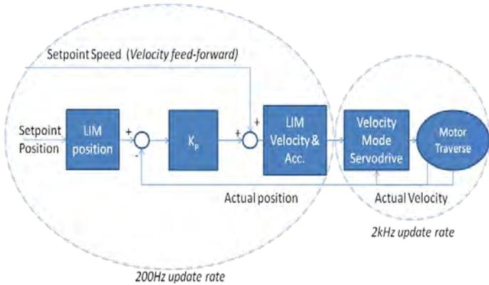
Figure 8: Control loop for linear actuator (LIM) steering
