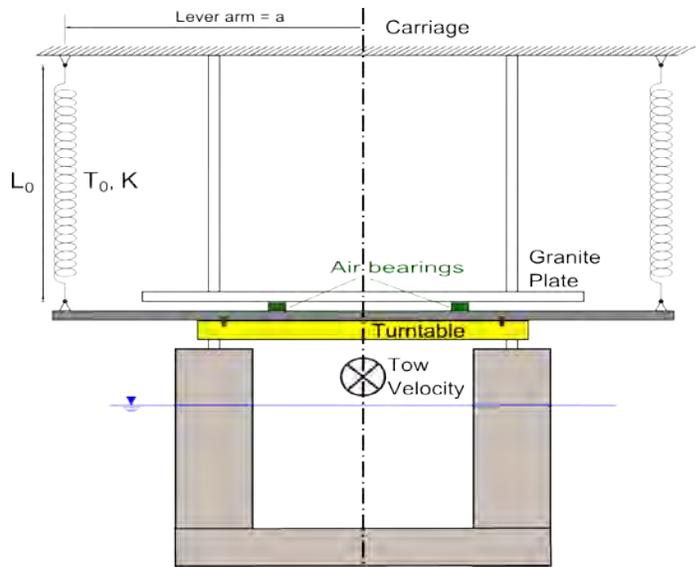
**Figure 4: Schematic of the experimental VIM test setup**
