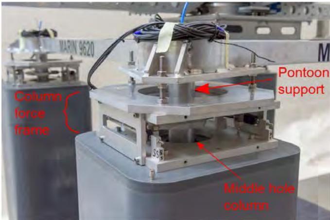
**Figure 2: Four column semi: three component column force frames and pontoon supporting frame**
