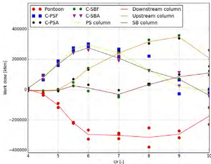
**Figure 14: Four column semi work done by columns and pontoon for 45 degrees heading and 10% damping**
