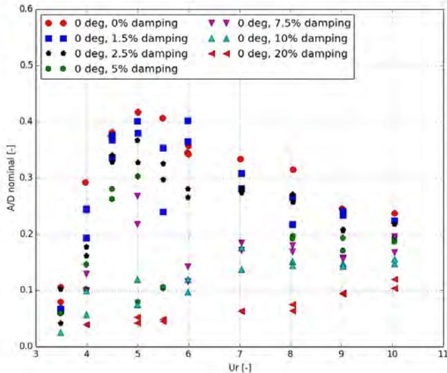
Figure 11: Paired-column semi nominal cross-flow amplitudes for 0 degrees heading
