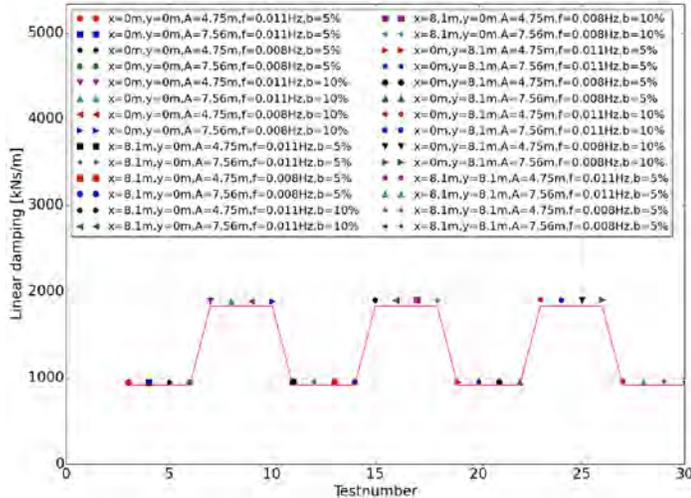
Figure 9: Overview results damping system integrity tests
