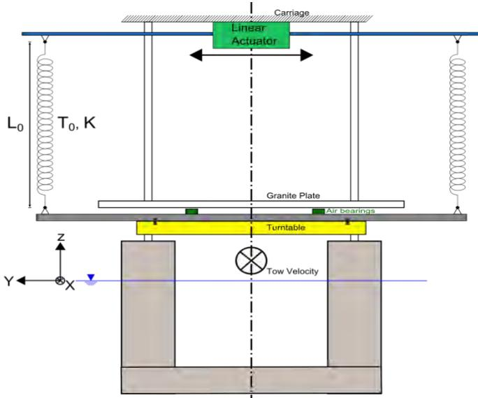
Figure 5: Schematic of the new experimental VIM test setup with optional cross-flow damping
