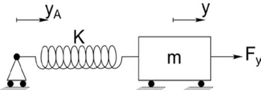
Figure 6 Simplified 1 DOF model of the active damping system, the mooring and the semi-submersible subjected to hydrodynamic loads.
