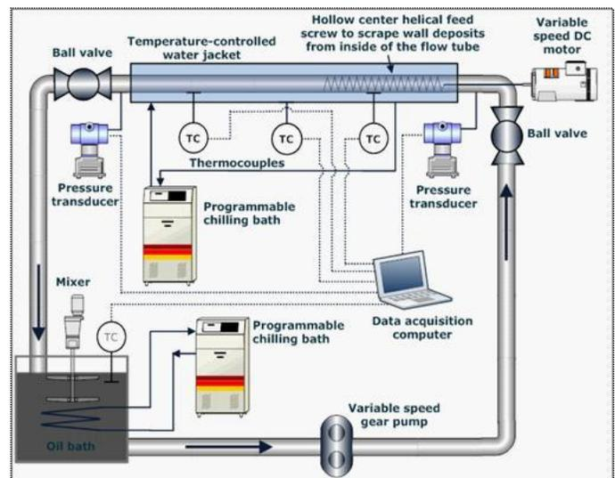
Schematic of the flow loop used in studying cold flow
