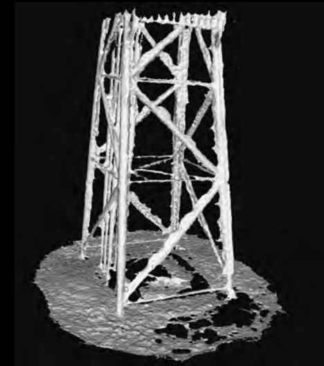
A 3D model data product of an offshore platform resulting from a Marlin System inspection. Photo credit: Lockheed Martin.
