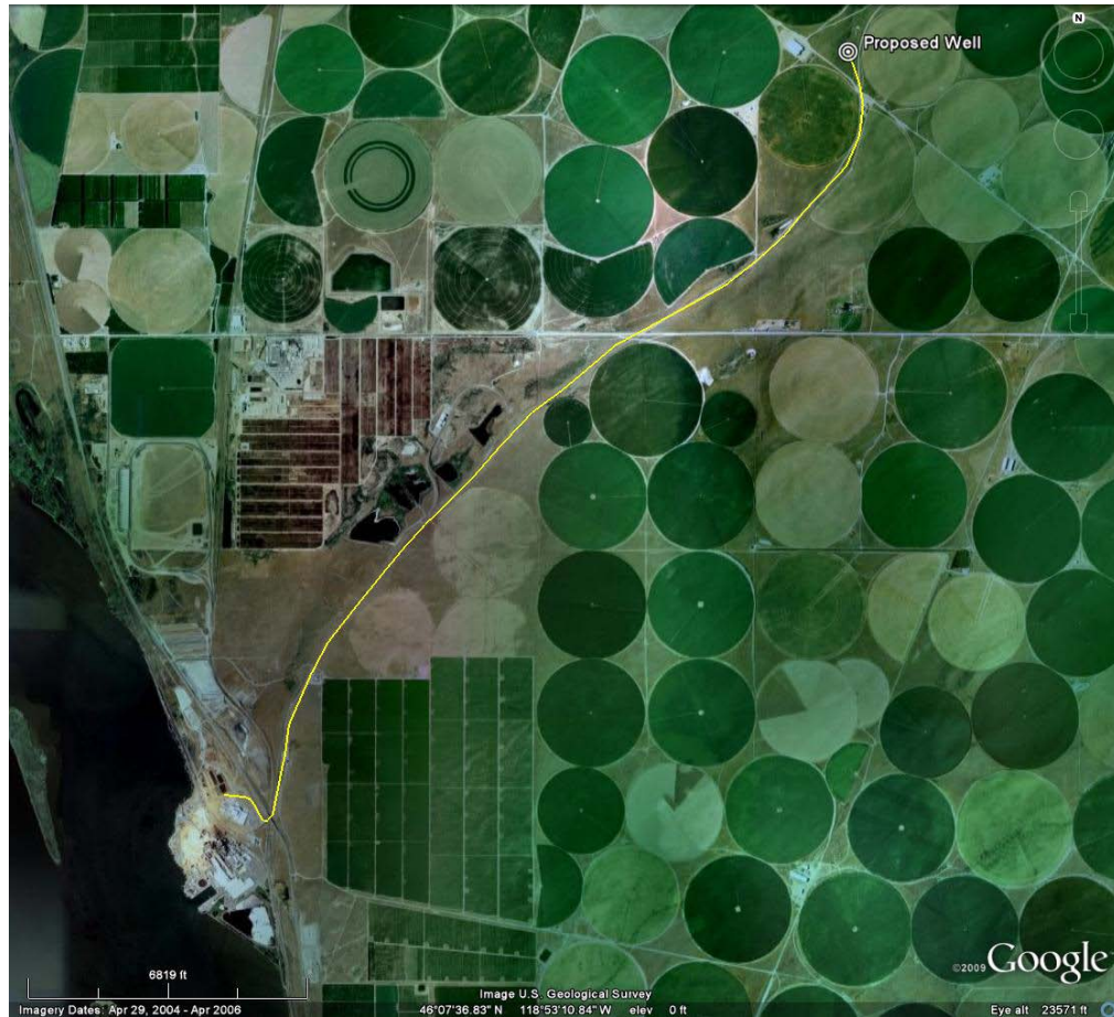
Figure 5.1. Proposed Pipeline Route to Sequestration Site. Total distance is 5 miles.
