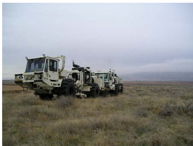
Figure 2.2. Two Vibroseis Trucks on Location at the Wallula Site
