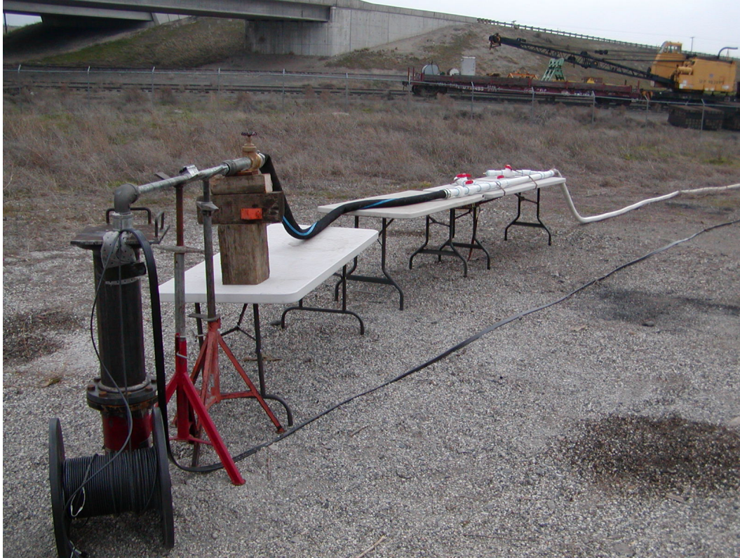
Figure C.2. Components of Surface Discharge Line and Conveyance System
