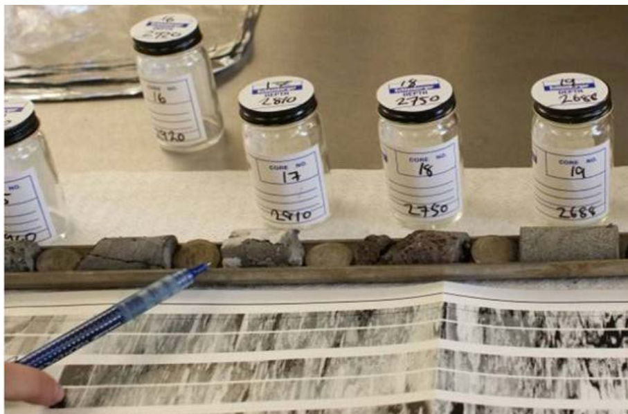
Figure 2.6. Rotary Sidewall Core Samples Shown as They were Examined at the Wellsite. Field print of the FMI allowed precise targetting of core samples.
