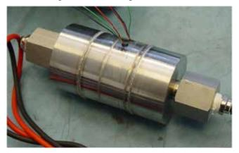
For the downhole application, this 2-inch diameter cell must be reduced to a cell and remote pressure diaphragms less than 0.75-inch in diameter. Fortunately, there remain numerous P and DP sensor chips in die-packs from the previous 1301 development, as shown in the example below.
