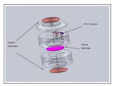
This oil-filled sensor cell was developed to extend the range of subsea flowmeters for operation in HP/HT conditions. The completed cell, shown in the following picture, was successfully tested at 250 deg C and 22,500 psi.
