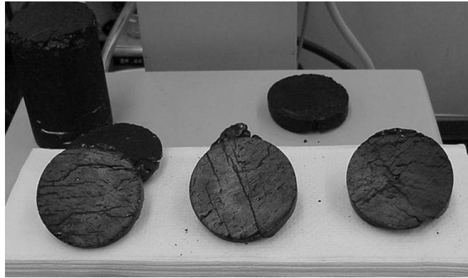
Figure 6. Photograph of trimmed ends from Gilson-seam coal cores 2 in. in diameter. Note the irregular cleat system associated with this coal.
