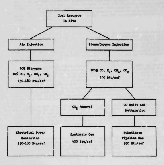
The Soviets have utilized the low Btu gas from air-blown gasification to generate electricity. Total gas production at Angrenskaya for 1963 (31 x 10° scf of -100 Btu/scf gas, some 2/3 of the Soviet in situ coal gasification production) was sufficient to produce more than 30 MWe of power. In comparison, for two one-month long periods the most recent Harna experiment produced gas at rates sufficient to generate 6.5 MWe: however, the gas was flared and not utilized.
