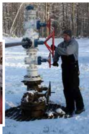
Injection well head
