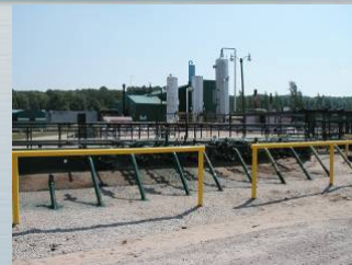
Active CO 2 EOR Flood with several additional wells present
