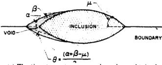
(e) The time-to-rupture curves have been obtained for the case when a polycrystal is deformed at a constant strain-rate at different temperatures. When no sliding of the boundaries is allowed then void nucleation is possible only when interface energies are comparable to the total surface energy of the void being created. These conditions may be met at non-wetting or almost non-wetting inclusions.
