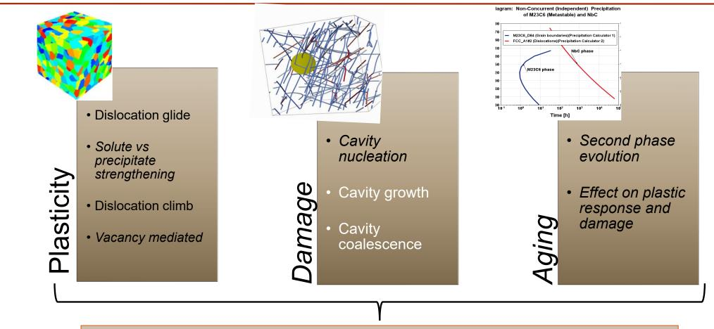
Effects of **microstructure** (grain size, texture, precipitates, dislocation content, solutes), **stress** (3D, time evolution), **temperature** (time evolution) on material performance
