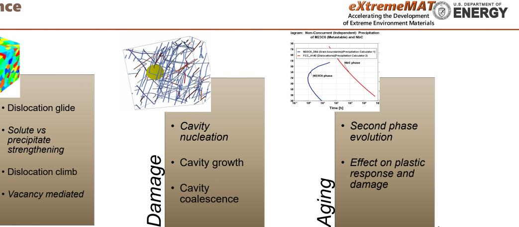
Effects of **microstructure** (grain size, texture, precipitates, dislocation content, solutes), stress (3D, time evolution), temperature (time evolution) on material performance
