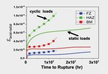
Using LaRomance (Los Alamos Reduced Order Models for Advanced Nonlinear Constitutive Equations), a surrogate model was developed for embedding into commercial finite element packages and can account for cyclical loading (demonstrated above for an idealized weld).
