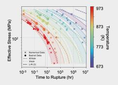
As demonstrated above for alloy P91, a rupture life criterion that considers uncertainty and is applicable to multi-axial loading was derived using limited experimental data.
