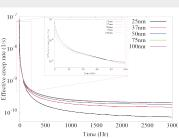
Simulation of carbide phase growth and dissolution during service and impact of carbide size on creep of type 347H stainless steel.
