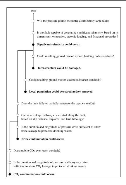
Figure 4: Event chain view of potential impacts from induced seismicity. The open channels (or gates) represent conditions that must be satisfied for the corresponding impact (indicated by the black dots) to occur. Active and passive safeguards can be introduced along the chain to reduce the likelihood of a given condition being satisfied, and therefore reducing overall risk.
