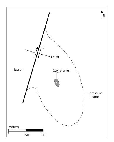
Figure 1: Pressure interaction between a CO<sub>2</sub> injector and a sealing fault.
