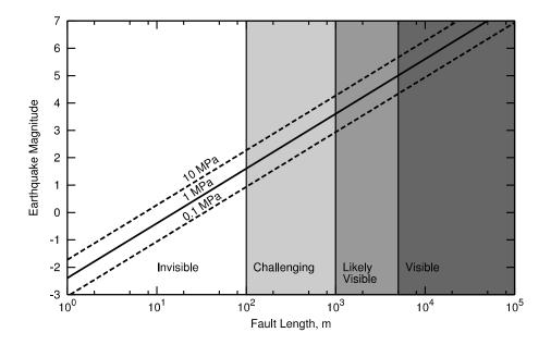
Figure 2: Theoretical relationship between fault rupture length (m), stress drop (MPa), and moment magnitude, assuming a circular rupture area. Shaded regions denote "typical" visibility of a fault of a given length using three-dimensional (3-D) seismic survey. Note that actual seismic resolution is highly specific to a given site and survey configuration, and should be carefully assessed.
