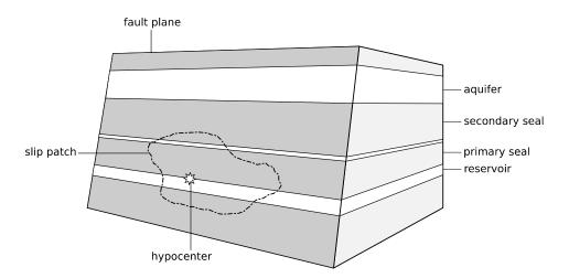
Figure 3: Cross-section along a fault plane that intersects a CO<sub>2</sub> storage reservoir and a shallow aquifer (vertical dimension not to scale). Increased pressure in the reservoir may trigger large-scale slip on the fault, and potentially open up a leakage pathway through the caprock seals.
