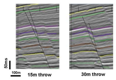
Figure 5: Example faults in surface seismic data with 15 m throw (left) and 30 m throw (right). Fault is solid black line with one splay fault interpreted. Figure from the Fault Analysis Group at University College Dublin (Fault Analysis Group, 2014).
