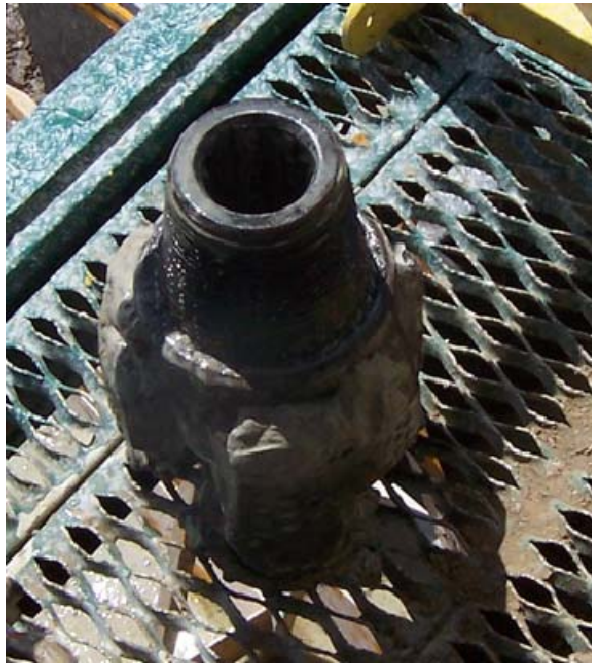
Figure 3-6. Photograph of Tricone Drill Bit Used to Drill the East Bend Well
