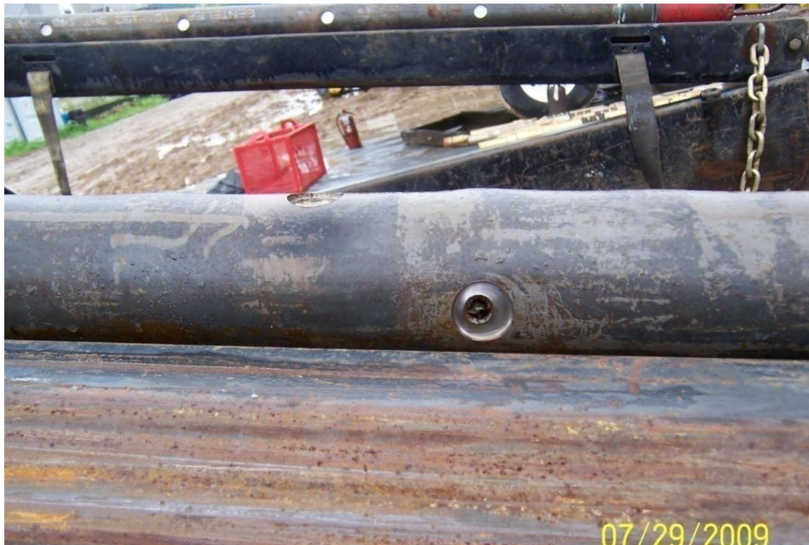
Figure 3-10. Photograph of Perforating Guns after being Fired
