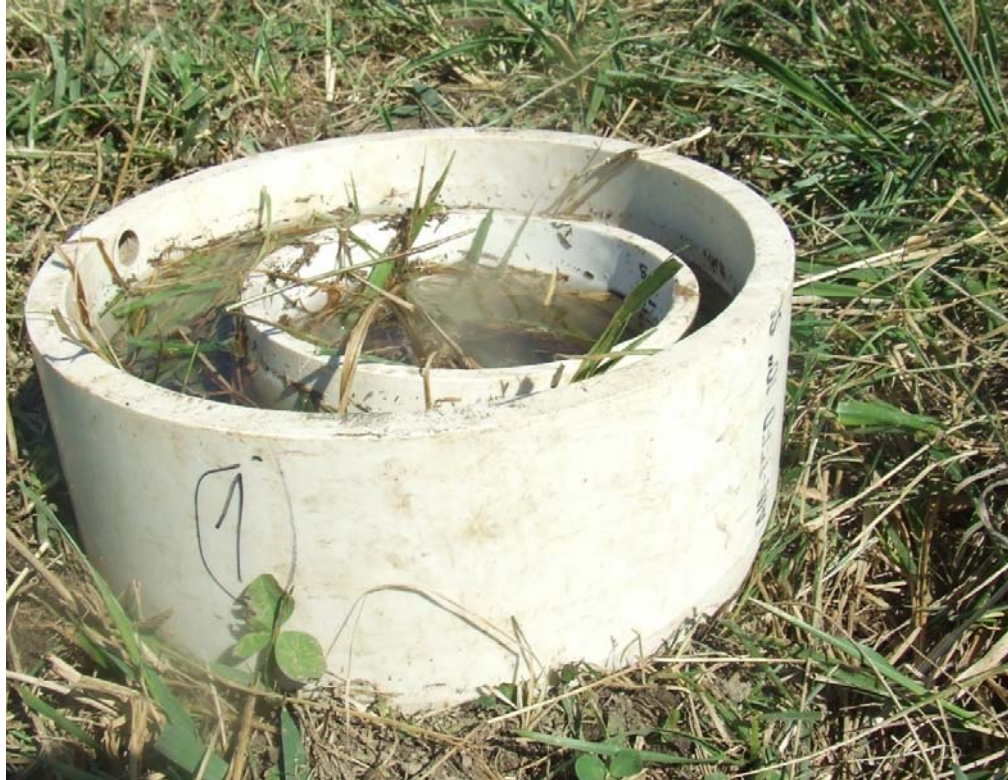
Figure 6. Double-Ring Infiltrometer, for Analyzing Soil Water Infiltration Under Field Conditions
