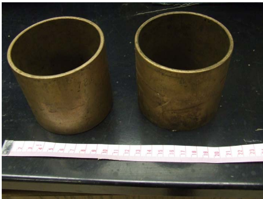
Figure 7. Cores for Analyzing Saturated Hydraulic Conductivity in the Laboratory Scale in cm
