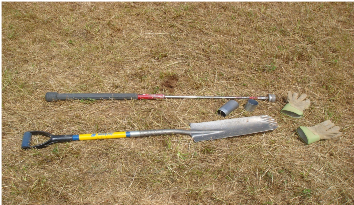
Figure 9. Tools (Shovel, Core Sampler, Gloves and Core) Used for Soil Core Sampling in the Field
