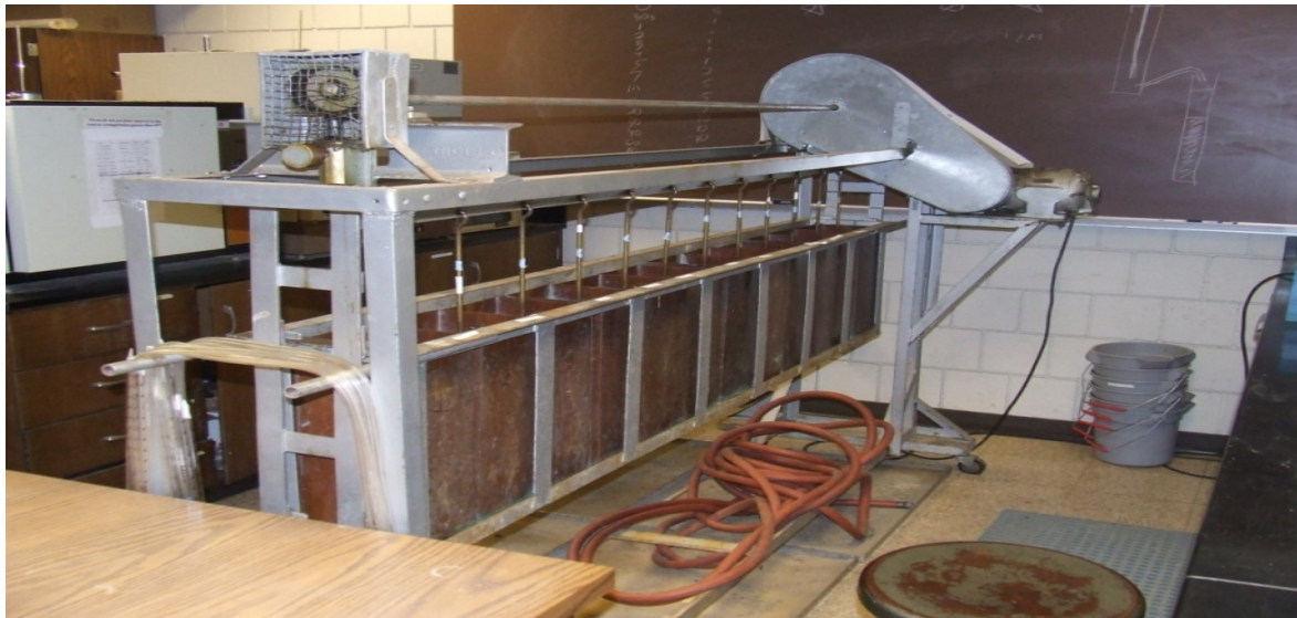
Figure 5. Wet Sieving Apparatus for Analyzing Aggregate Size Distribution, and Stability
