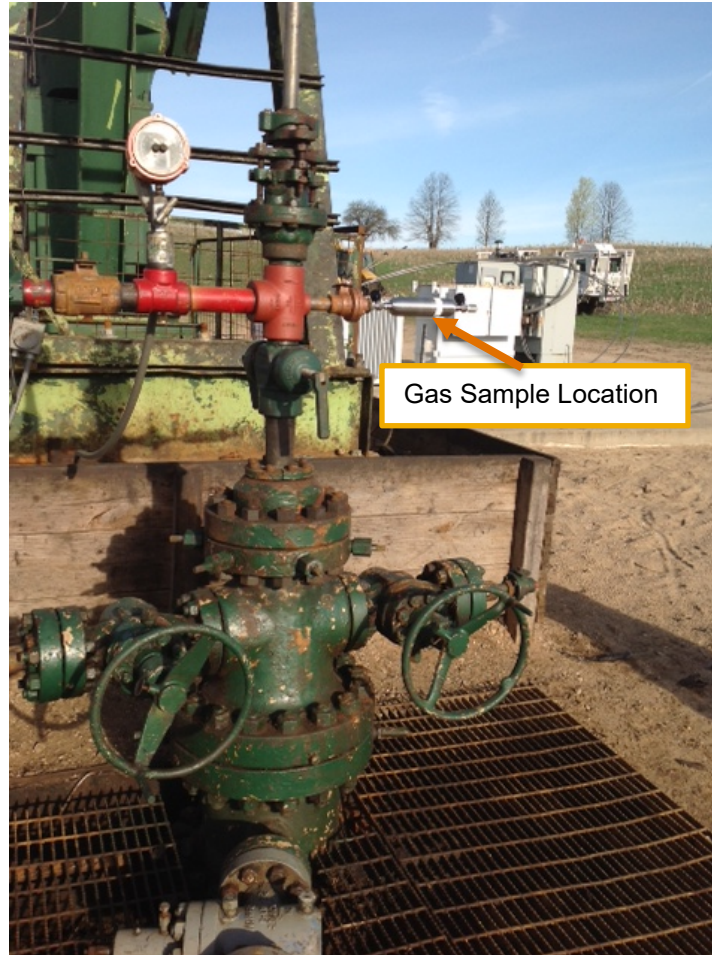
Figure 2-2. Collection of a Gas Sample from the Well Tubing.
