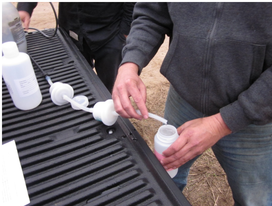
Figure 2-1. Preparation (Filtering) of the Brine Samples.
