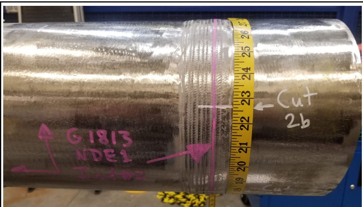
Image 4 (G1813-NDE1 Circumferential Indication 2 - Cut Location 2b)
